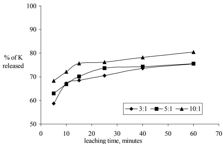
Fig. (1) Percent of K released in the water/CKD leachates at 30 °C and different liquid:solid weight ratios.
