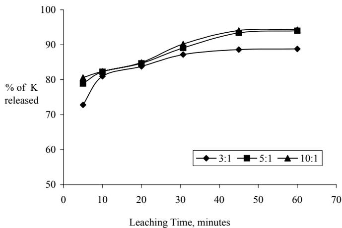
Fig.(6): Percentage of K released in calcium nitrate solution/CKD leachates at 50 °C and different liquid:solid weight ratios.
