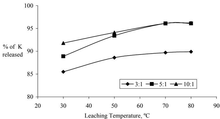
Fig(10):Percentage of Potassium released in the Calcium Nitrate solution/CKD leachates after the initial 45 minutes of leaching at different temperatures and liquid : solid weight ratios.
