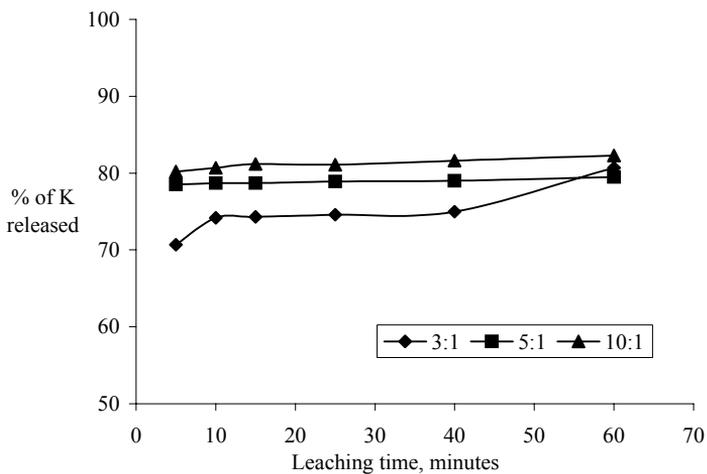
Fig.(4) Percent of K released in the water/CKD leachates at 80 °C and different liquid:solid weight ratios.
