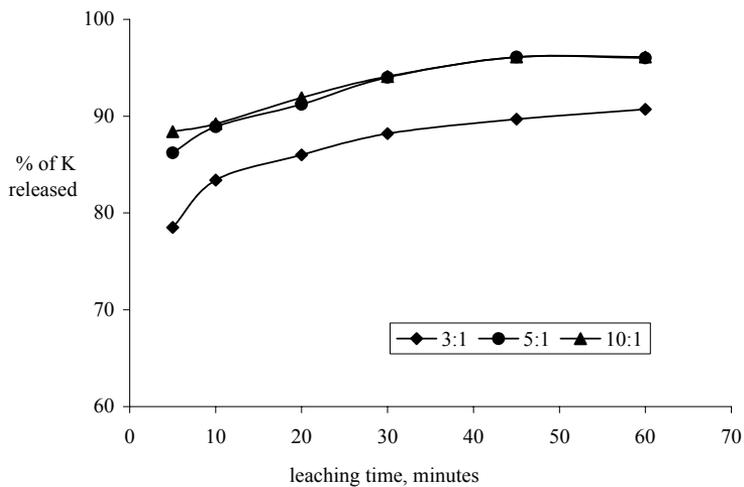
Fig.(7): Percentage of K released in calcium nitrate solution/CKD leachates at 70 °C and different liquid : solid weight ratios.
