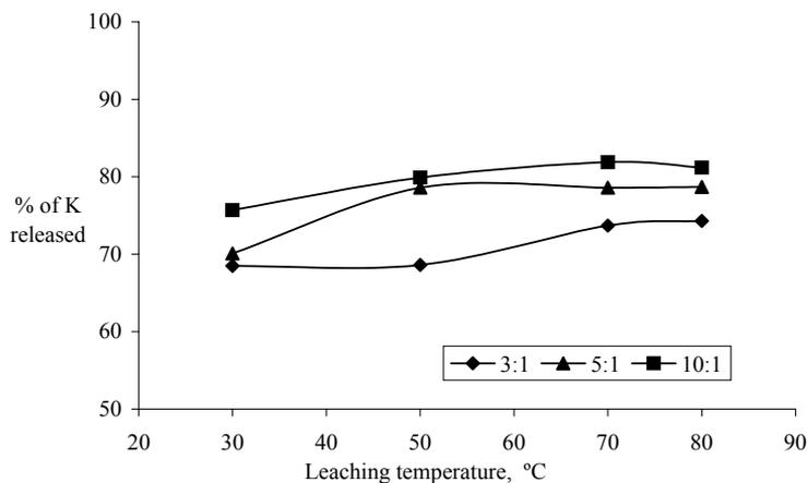
Fig (9):Percent of Potassium released in the water/CKD leachates after the initial 15 minutes of leaching at different temperatures and liquid : solid weight ratios.
