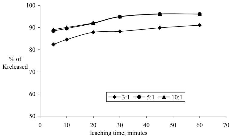
Fig.(8): Percentage of K released in calcium nitrate solution/CKD leachates at 80 °C and different liquid : solid weight ratios.
