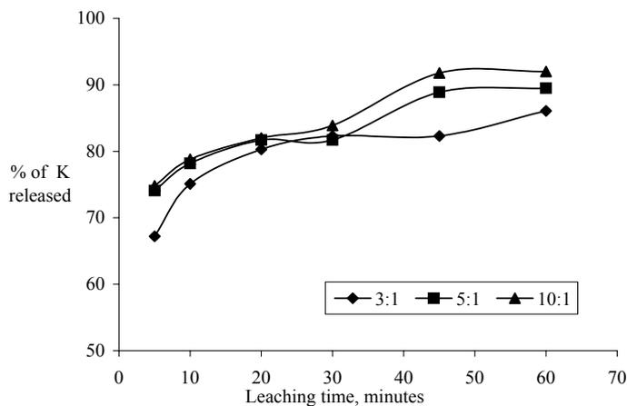
Fig.(5): Percentage of K released in calcium nitrate solution/CKD leachates at 30 °C and different liquid:solid weight ratios.
