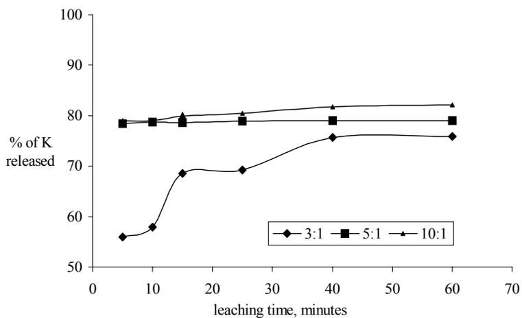
Fig. (2) Percent of K released in the water/CKD leachates at 50 °C and different liquid:solid weight ratios.
