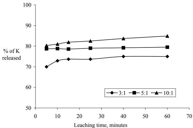
Fig.(3) Percent of K released in the water/CKD leachates at 70 °C and different liquid:solid weight ratios.
