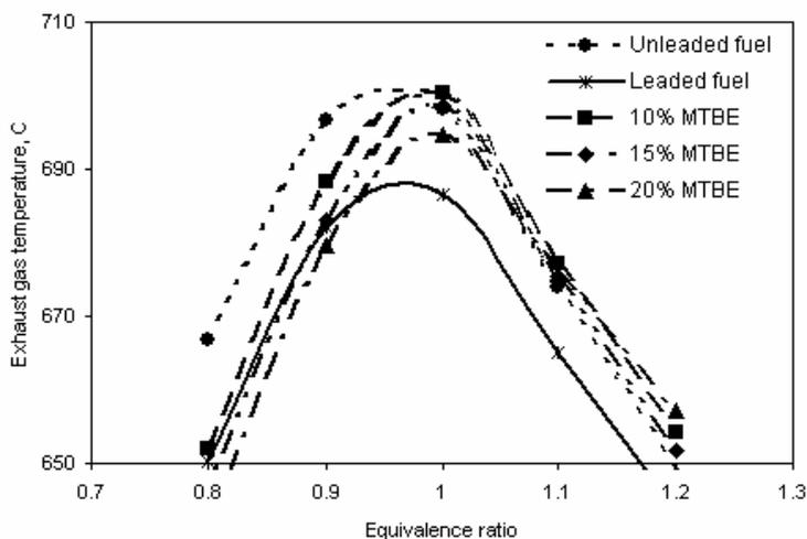
Fig. 1: The effect of equivalence ratio on the exhaust gas temperature
