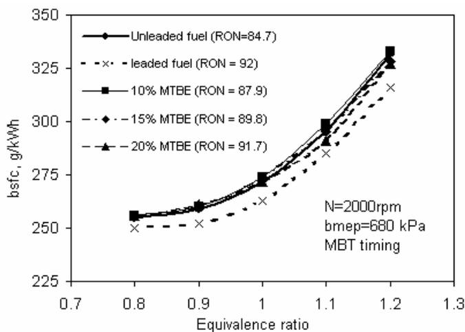
Fig. 2: The effect of equivalence ratio on the engine bsfc
