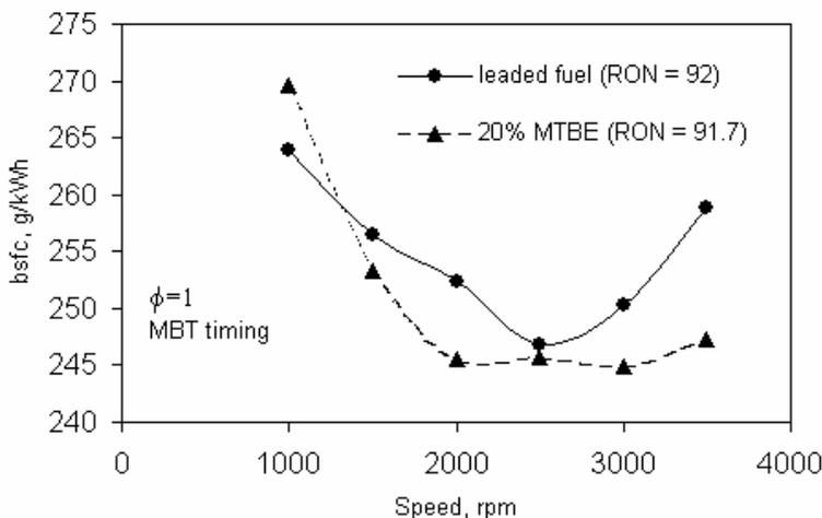
Fig. 3: The effect of engine speed on the engine bsfc
