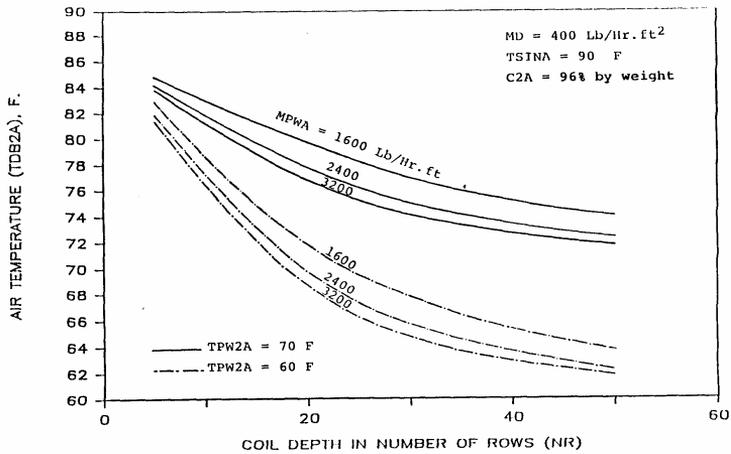
Figure 7: Temperature of air leaving the absorber versus packing depth, for different cooling water flow rates and inlet
