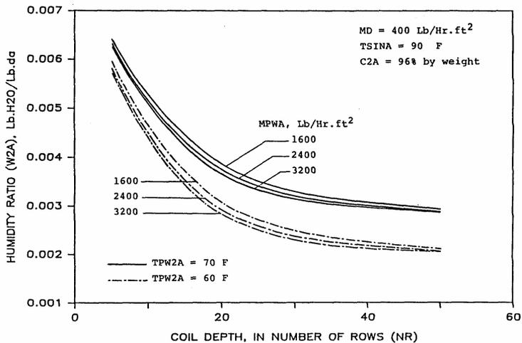
Figure 8: Humidity ratio of air leaving the absorber, versus packing depth, for different cooling water flow rates and inlet temperatures
