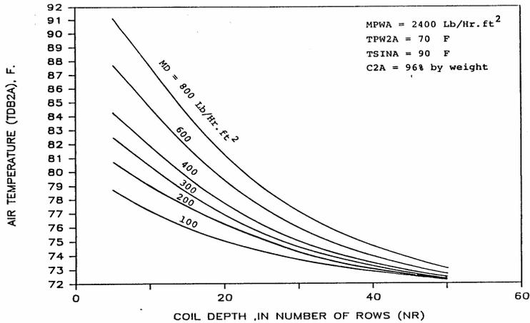
Figure 3: Temperature of air leaving the absorber versus packing depth, for different desiccant flow rates.
