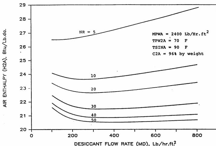
Figure 4: Enthalpy of air leaving the absorber, versus desiccant flow rates, for different packing depths
