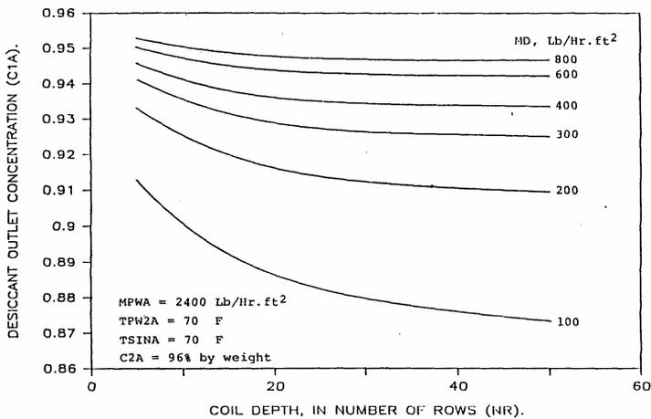
Figure 6: Concentration by weight of the desiccant solution leaving the absorber versus packing depth, for different desiccant flow rates
