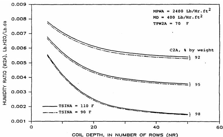
Figure 10: Humidity ratio of air leaving the absorber, versus packing depth, for different desiccant solution inlet concentrations and temperatures
