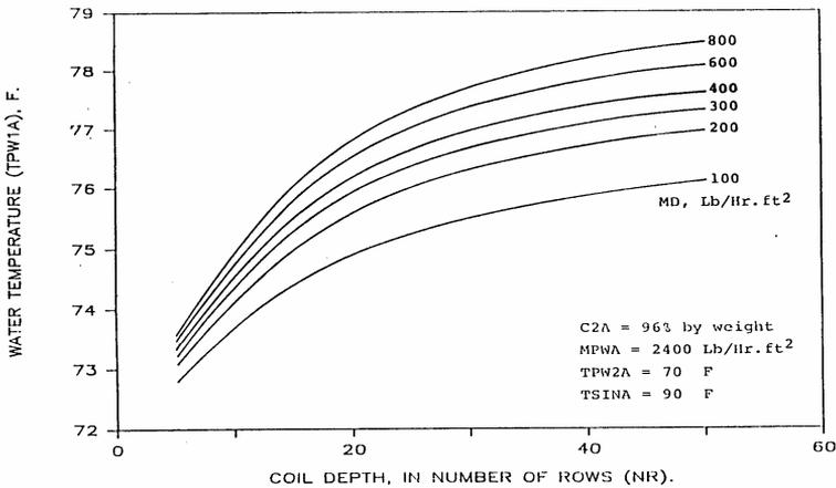
Figure 5: Outlet temperature of cooling water, versus packing depth, for different desiccant flow rates.
