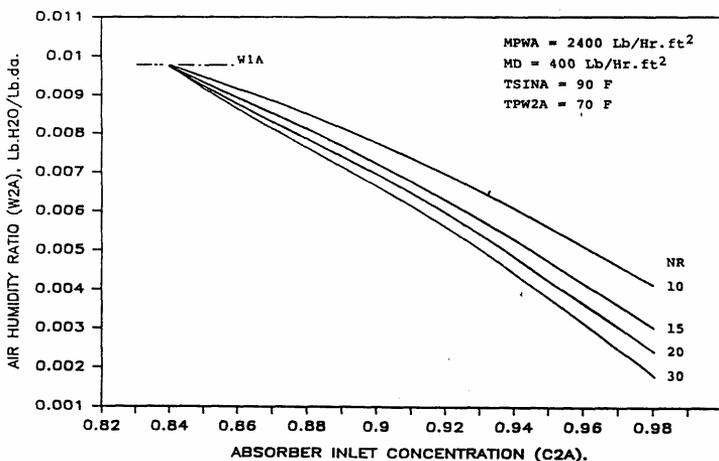
Figure 11: Humidity ratio of air leaving the absorber, versus desiccant solution inlet concentrations, for different packing depths
