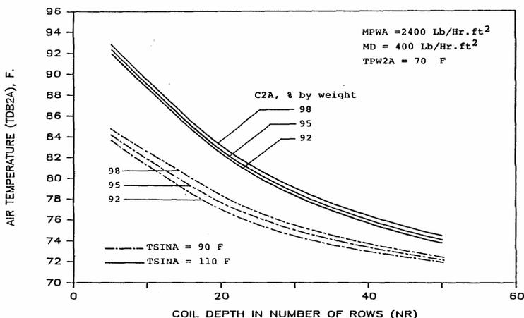
Figure 9: Temperature of air leaving the absorber, versus packing depth, for different desiccant solution inlet concentrations and temperatures.
