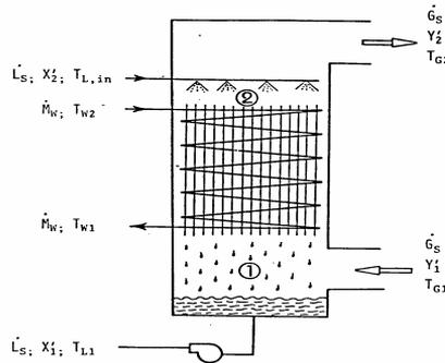
Figure 1: Non- adiabatic column packed with finned-tube heat exchangers.
