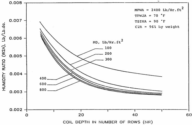
Figure 2: Humidity ratio of air leaving the absorber, versus packing depth, for different desiccant flow rates
