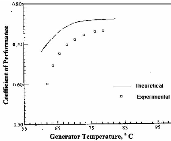
Figure (6) Experimental Data for the System C.O.P vs. the Generator Temperature
