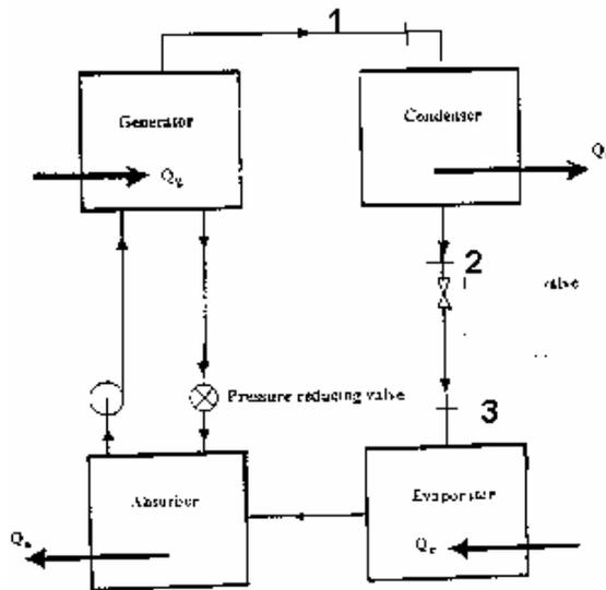
Figure (1) Simple Diagram for an Absorption Refrigeration System
