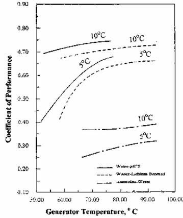
Figure (3) A Comparison between the Performances of the three refrigerant systems [H<sub>2</sub>O-NH<sub>3</sub>, (MCS)-H<sub>2</sub>O and LiBr-H<sub>2</sub>O].as a Function of the Evaporator Temperature.
