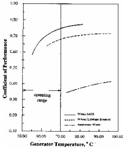
Figure (4) Suggested Operating Range for the Selected Water-MCS Solution as a Working Fluid
