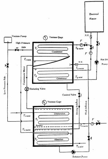
Figure (5) Experimental Setup of the Single-Stage Single-Effect Absorption System
