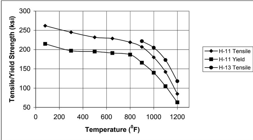
**Figure-6** Variation of tensile strength ( $\sigma_u$ ) and yield strength ( $\sigma_y$ ) with temperature for H-11 and H-13 hot work tool steels.
