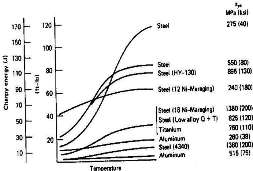
Figure-1 Transition behavior evidenced from variation of Charpy impact energy against temperature for several engineering alloys [Hertzberg, 1996].
