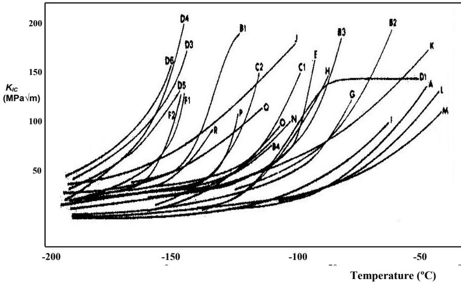
**Figure 7** Variation of  $K_{IC}$  with temperature for various steels studied by Marandet and Sanz [1977].
