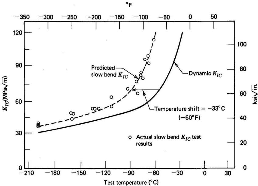
**Figure-4** (a) Use of *CVN* test results to predict the effect of loading rate on  $K_{IC}$  for strain-rate sensitive A517-F steel [Barsom and Rolfe, 1970].
