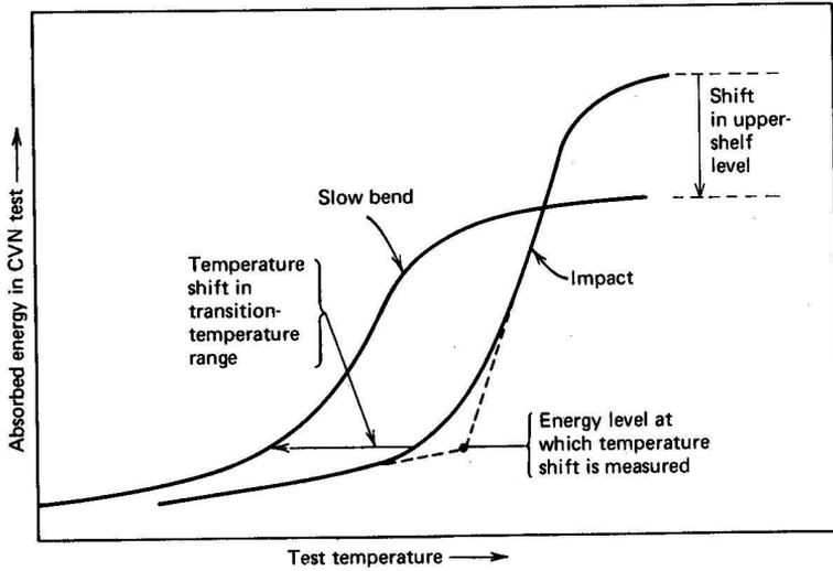
**Figure-3** Impact energy versus test-temperature, showing shift in transition-temperature due to change in strain-rate [Barsom and Rolfe, 1970].
