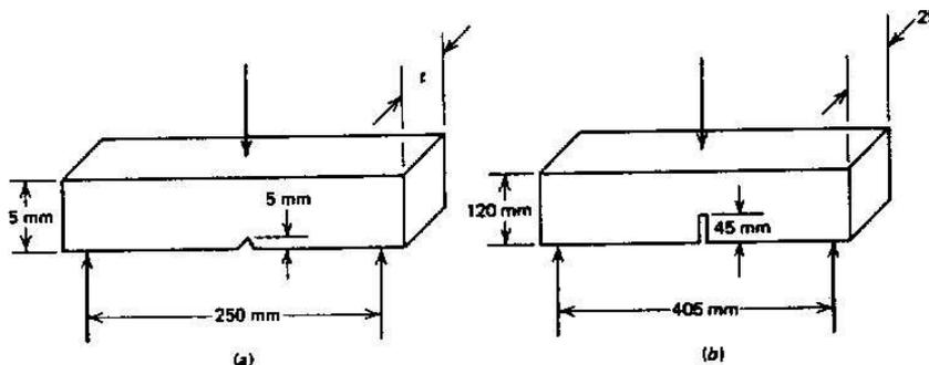
Figure-2 (a) Drop-weight tear test (DWTT) specimen with shallow notch pressed into bar; (b) Dynamic tear test (DT) specimen with machined slot introduced into titanium-embrittled electron beam weld [Hertzberg, 1996].
