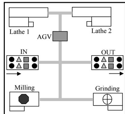
Figure 1. A Flexible Manufacturing Cell
