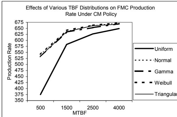
Figure 7. Effects of Various Failure Distributions on FMC Production Rate.
