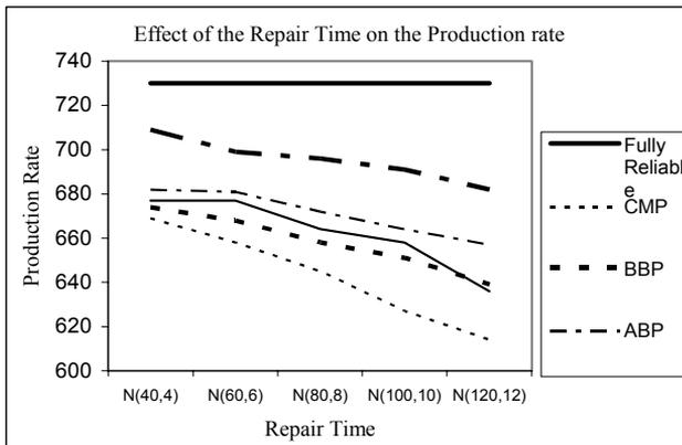
Figure 5. Effects of Repair Time on FMC Production Rate
