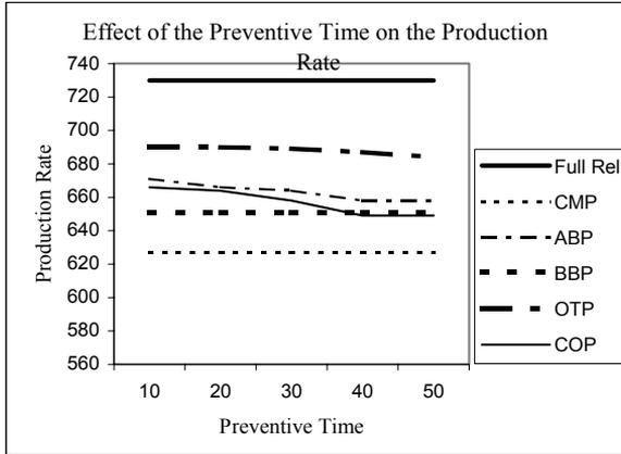
Figure 4. Effects of variable PM time on FMC production rate
