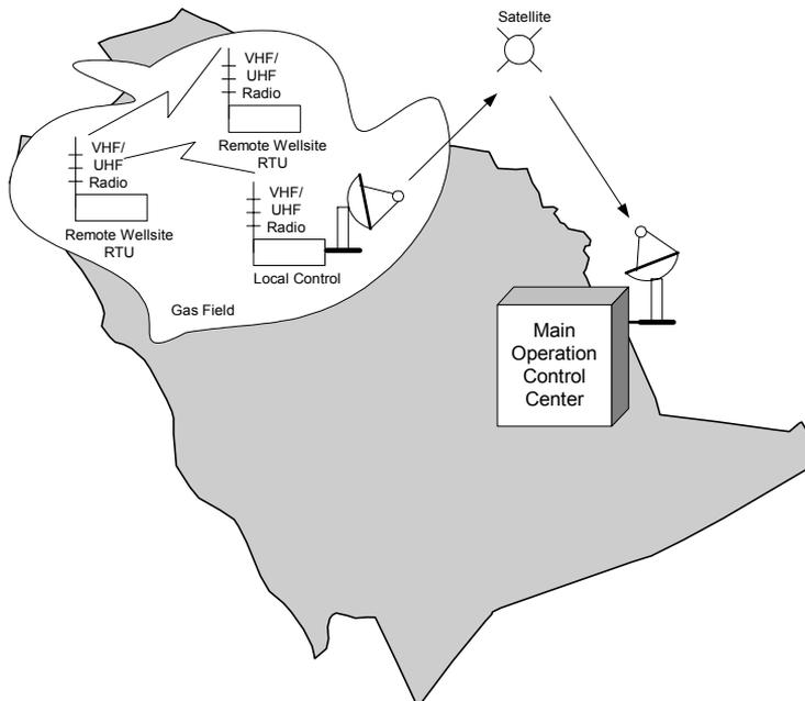
FIGURE III: SCADA COMMUNICATIONS EXAMPLE
