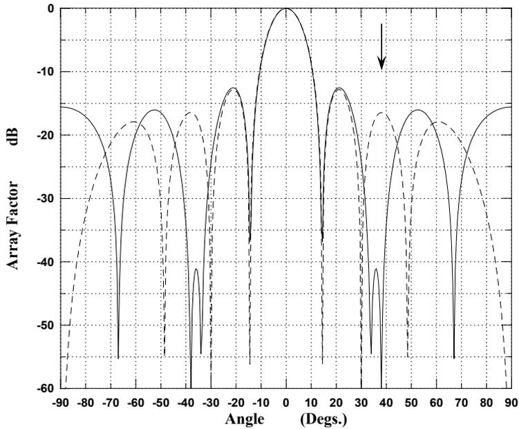
Figure (2-a) Array pattern of an 8 element uniform array with  $d = 0.5\lambda$  (dashed). The main beam is at  $\theta_s = 0^\circ$ . One null is imposed at  $\theta_m = 38^\circ$  (solid) using genetic algorithms.
