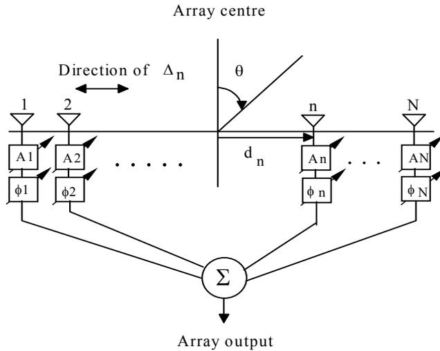
Figure (1) The linear array geometry
