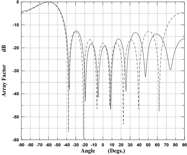
Figure (3) Array pattern of an 8 element uniform array with  $d = 0.5 \lambda$ . The main beam is at  $\theta_s = -60^\circ$  (dashed). Array pattern is restricted to  $-15$  dB at  $\theta_m = 55^\circ, 75^\circ, 90^\circ$  using genetic algorithms (solid).
