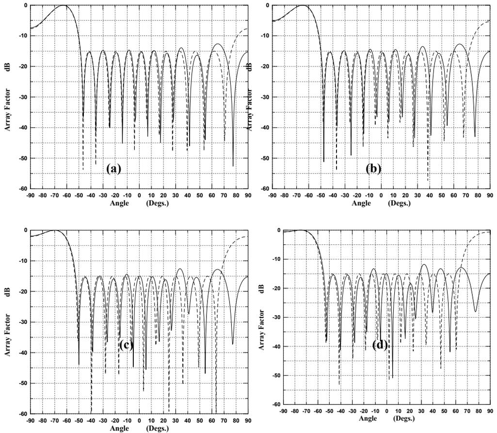
Figure (5) Array pattern of a 12 element 15 dB Chebyshev scanning array with  $d = 0.5 \lambda$ . The main beam is at: (a)  $\theta_s = -63^\circ$ , (b)  $\theta_s = -65^\circ$ , (c)  $\theta_s = -70^\circ$ , and (d)  $\theta_s = -75^\circ$  (dashed). Array pattern is restricted to -15 dB at  $\theta_m = 50^\circ, 60^\circ, 75^\circ, 90^\circ$  using genetic algorithms (solid).
