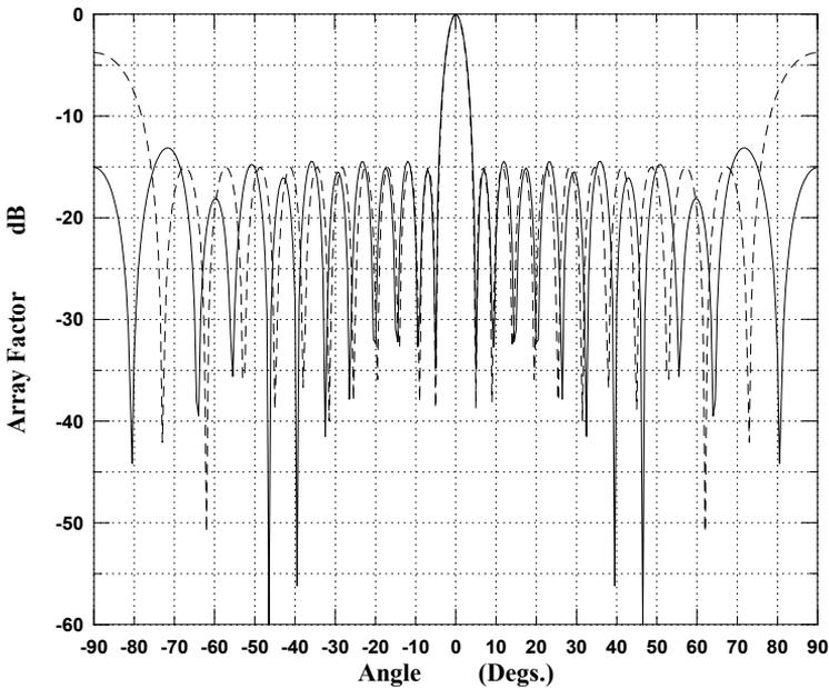
Figure (4) Array pattern of a 12 element 15 dB Chebyshev array with  $d = 0.96 \lambda$ . The main beam is at  $\theta_s = -60^\circ$  (dashed). Array pattern is restricted to  $-15 \text{ dB}$  at  $\theta_m = 50^\circ, 75^\circ, 90^\circ$  using genetic algorithms (solid).
