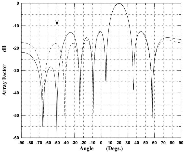
Figure (2-b) Array pattern of an 8 element uniform array with  $d = 0.5\lambda$ . The main beam is at  $\theta_s = 20^\circ$  (dashed). One null is imposed at  $\theta_m = -50^\circ$  (solid) using genetic algorithms.
