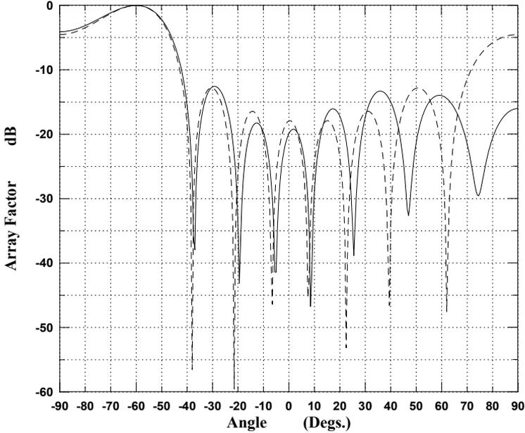
Figure (3) Array pattern of an 8 element uniform array with  $d = 0.5 \lambda$ . The main beam is at  $\theta_s = -60^\circ$  (dashed). Array pattern is restricted to  $-15 \text{ dB}$  at  $\theta_m = 55^\circ, 75^\circ, 90^\circ$  using genetic algorithms (solid).
