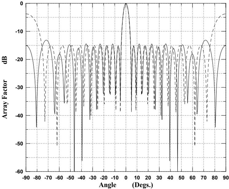
Figure (4) Array pattern of a 12 element 15 dB Chebyshev array with  $d = 0.96 \lambda$ . The main beam is at  $\theta_s = -60^\circ$  (dashed). Array pattern is restricted to  $-15$  dB at  $\theta_m = 50^\circ, 75^\circ, 90^\circ$  using genetic algorithms (solid).
