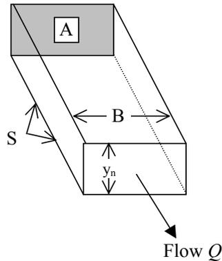
Under uniform flow conditions, the flow is calculated by the following relationship, based on Manning's equation
