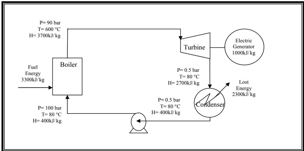
Figure-2: Cogeneration Cycle
