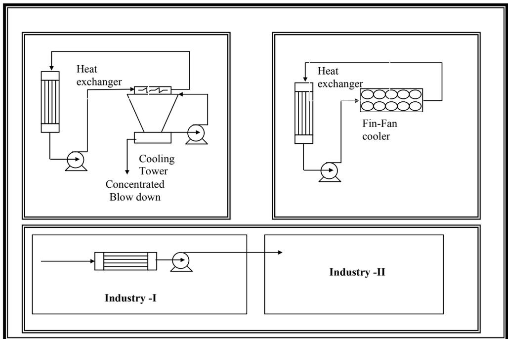
Figure-3: Once Through Cooling System
