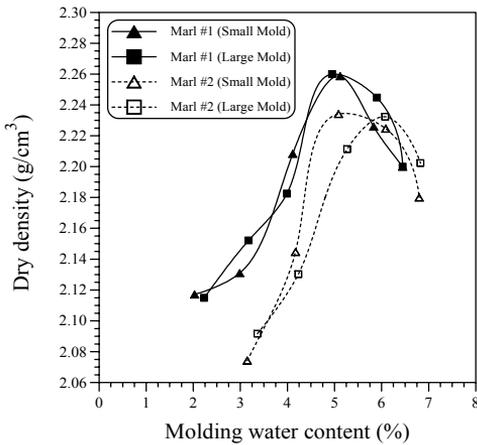
Figure 7. The moisture-density relationships for both marls using both molds
