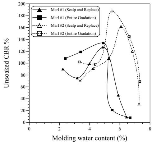
Figure 8. The CBR-moisture relationships for both marls using the large mold
