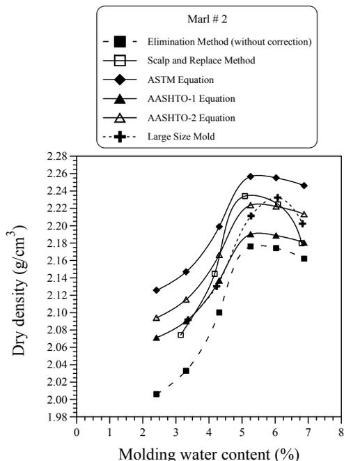
Figure 13. The moisture-density relationships for Marl #2 using different correction methods
