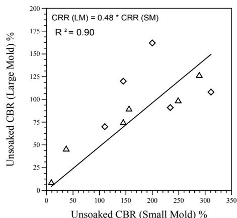
Figure 10. The correlation between the CBR values obtained using both molds for both marls
