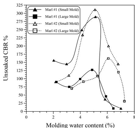
Figure 9. The CBR-moisture relationships for both marls using the conventional and large size molds
