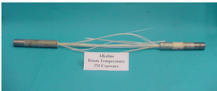
Figure 2. Typical failure mode of GFRP bar in tension.
