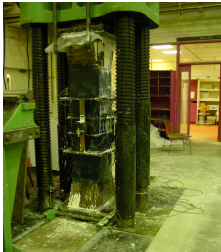
Figure 5. Test setup for column specimen of second series specimens.
