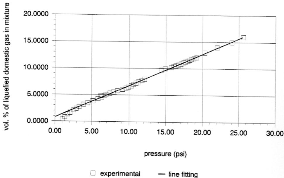
Figure 5: relation between gas pressure and vol.% of liquefied domestic gas in acetic acid/n-pentane mixture
