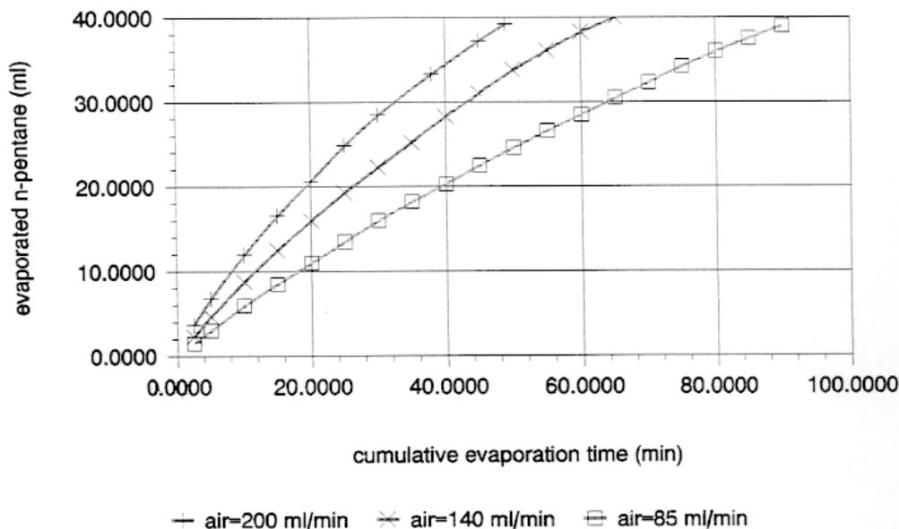
Figure 8: evaporation rate of n-pentane from a mixture of 40% V/V with acetic acid by air bubbling
