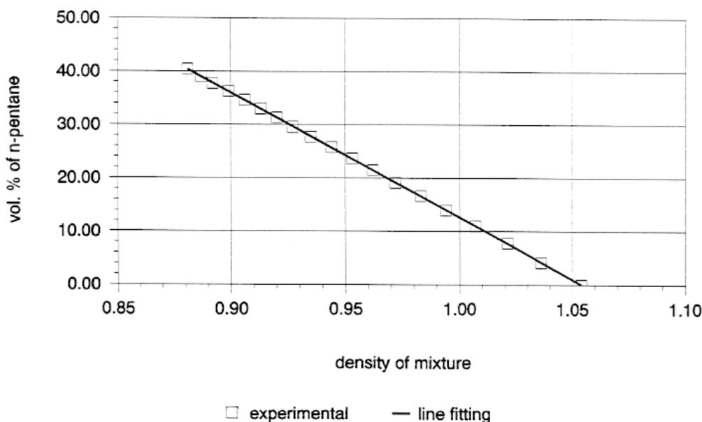
Figure 2: change of density with vol.% of n-pentane in acetic acid/n-pentane mixture
