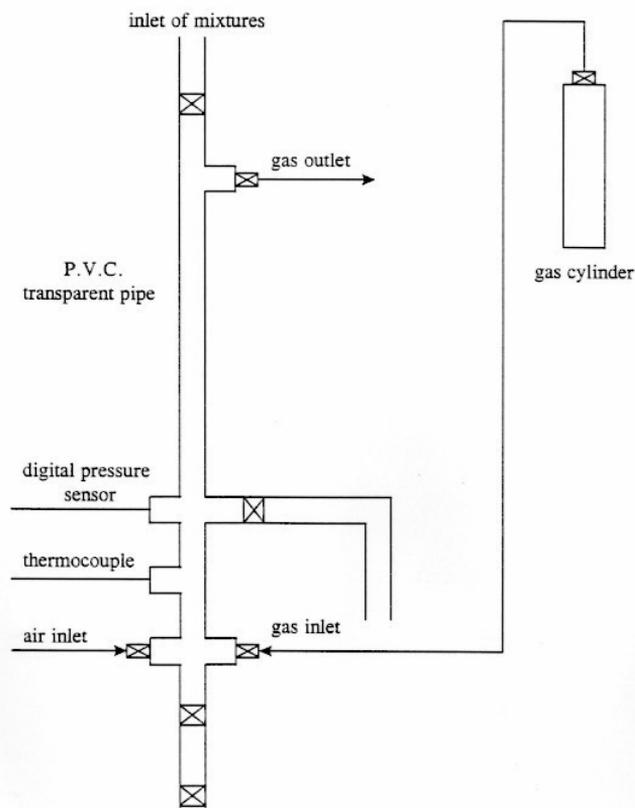
Figure 1 : experimental rig
