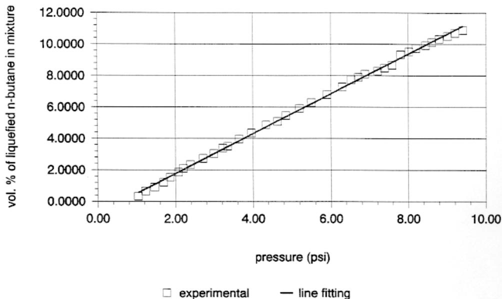
**Figure 3: relation between gas pressure and volume % of liquefied n-butane in its mixture with acetic acid and n-pentane**
