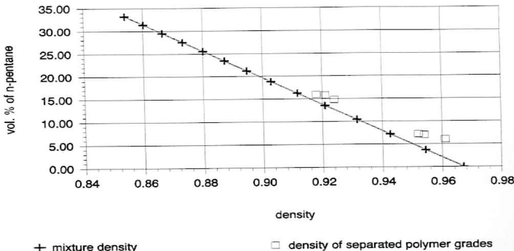
Figure 9: separation of polymer pellets with vol.% n-pentane in its mixture with tetralin
