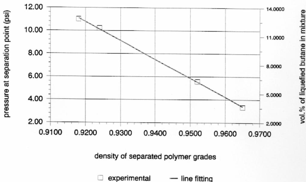
Figure 4: separation points of polyethylene pellets during addition of liquefied n-butane gas to acetic acid/n-pentane mixture
