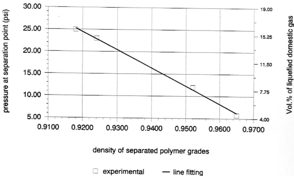
Figure 6: Separation points of polyethylene pellets during addition of liquefied domestic gas to acetic acid/n-pentane mixture
