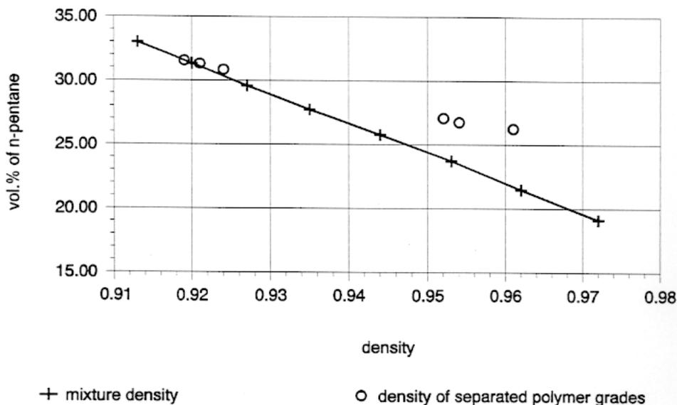
Figure 7: separation of polymer pellets with vol.% n-pentane in its mixture with acetic acid
