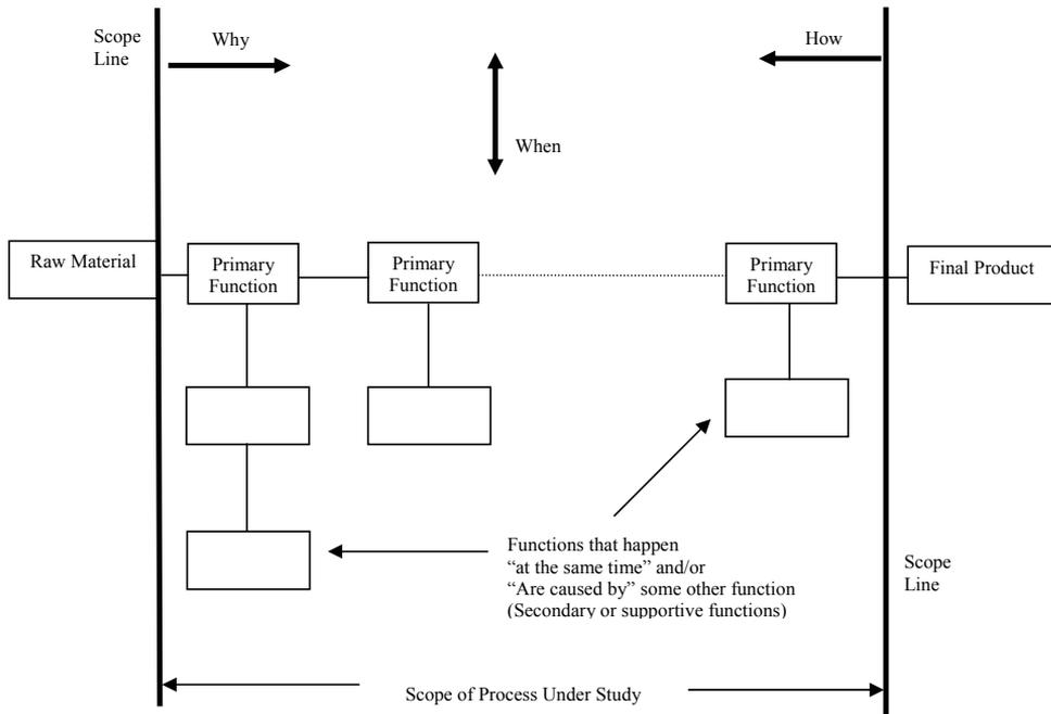
Figure 1: Process Functional Analysis System Techniques Diagram
