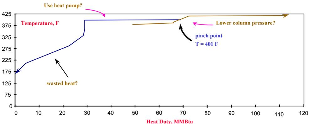
Figure 8: Pinch Diagram for Case Study 2
