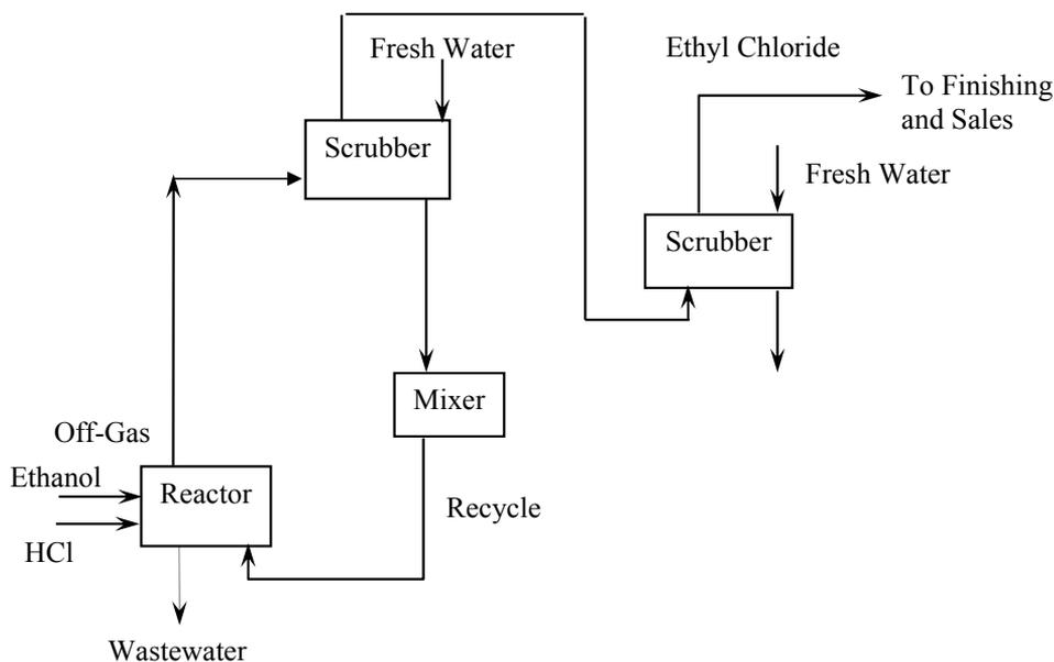
Figure 2: Ethyl Chloride Process
