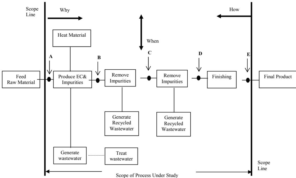
Figure 3: Process Functional Analysis System Techniques Diagram
