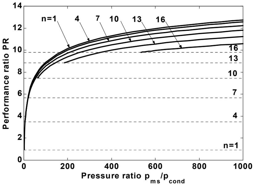
Figure 9. Comparison of performance ratio of a MED unit with and without thermal compressor
