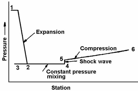
Figure 4. Pressure at the different stations of a steam ejector
