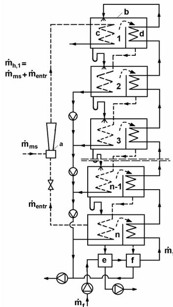
**Figure 1. A schematic of the studied system of MED unit with thermal compressor**
