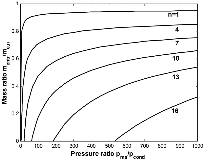
Figure 8. Dependence of the mass flow ratio of entrained vapor and released vapor in the last effect on motive steam pressure
