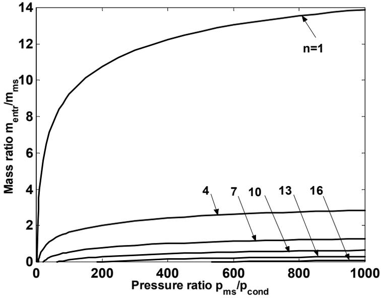
Figure 7. Effect of motive steam pressure on the mass flow ratio of entrained vapor and motive steam
