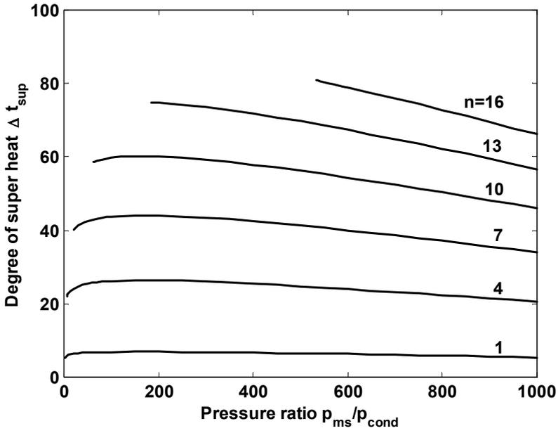
Figure 6. Dependence of superheat degree of the heating vapor in the first effect on the motive steam pressure
