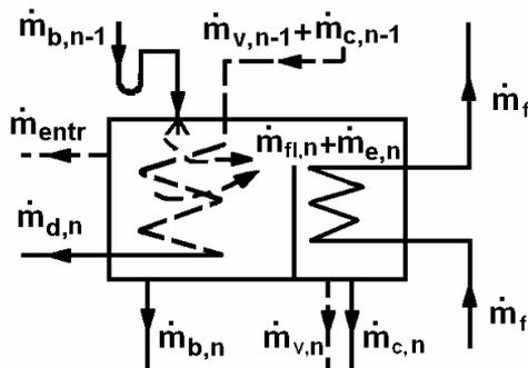
Figure 2. Mass flow rates of brine, steam, vapor, condensate and distillate in the effects of the studied system
