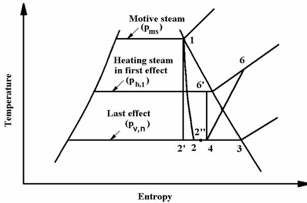
Figure 5. Representation of the steam and water vapor at the different stations of the steam ejector on T-s diagram
