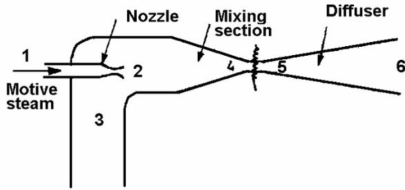
Figure 3. A Section through a steam ejector
