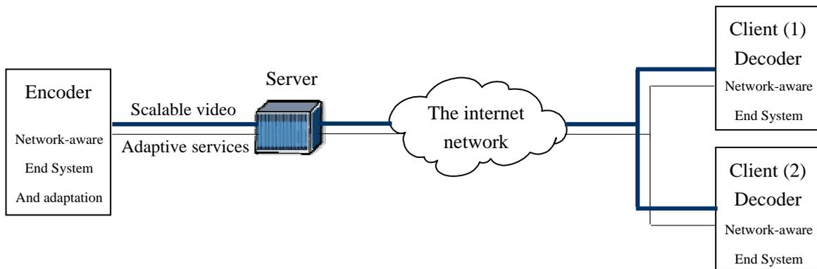
Fig. 1 System configuration for internet streaming of video
