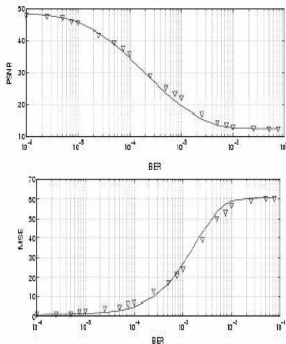
Fig.5 Image quality versus channel bit error ratio
