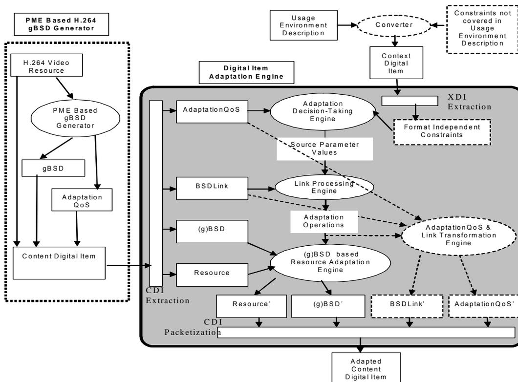
Fig.6 System Architecture of PME based H.264 video adaptation for Digital Item Adaptation
