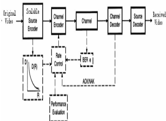
Fig. 4 System architecture of Joint Source-Channel Coding for wireless video transmission
