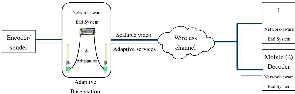
Fig. 2 System configuration for video streaming over cellular mobile network
