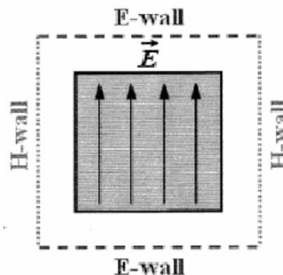
Figure 2- Equivalent unit cell for an infinite array of equal size patches
