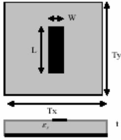
Figure 3- The unit cell of a microstrip dipole infinite array.
