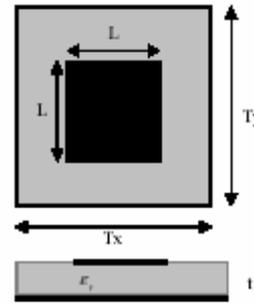
Figure 5- The unit cell of a square patch infinite array
