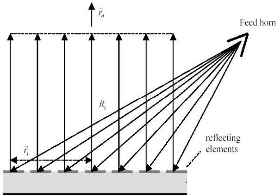
Figure 1. A microstrip reflectarray antenna
