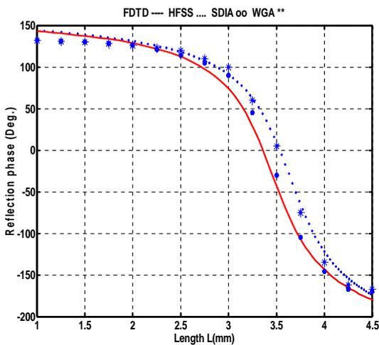
Figure 4- Phase response of a microstrip dipole infinite array
