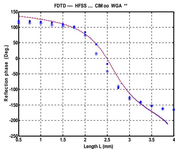
Figure 6- Phase response of square patch infinite array
