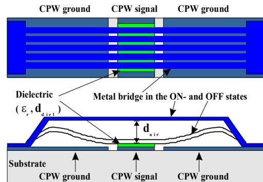
Fig.1: Standard RF-MEMS capacitive shunt switch
