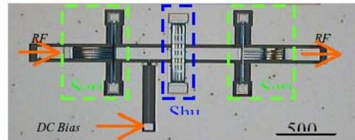
Fig.9: Series-Shunt-Series architecture including biasing circuit and pad.
