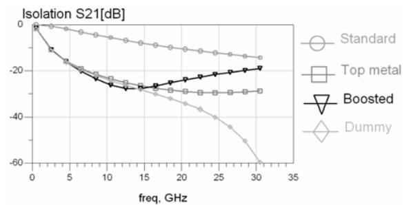
Fig.7b: Isolation Loss Measurements
