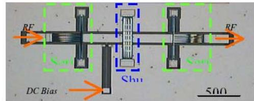
Fig.9: Series-Shunt-Series architecture including biasing circuit and pad.
