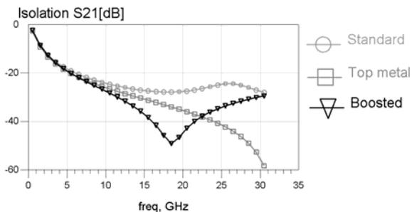
Fig.6b: Simulated HFSS Isolation of standard switch, switch with floating top metal, boosted switch.
