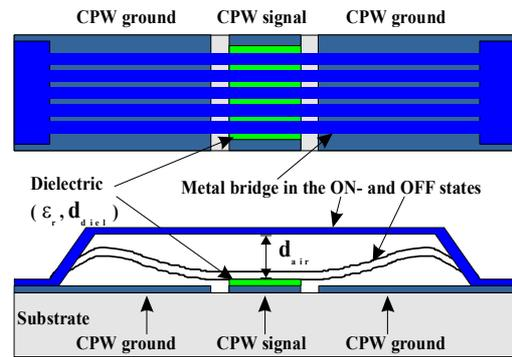
Fig.1: Standard RF-MEMS capacitive shunt switch
