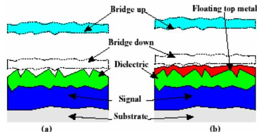
Fig.2: Close-up on the active area showing the parasitic air-gaps as a result of the surface roughness: a) conventional, b) with floating metal
