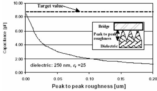
Fig.3: Influence of the roughness on the down capacitance
