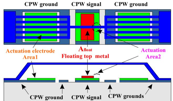
Fig.4: MEMS switch implementing a floating top metal covering the dielectric
