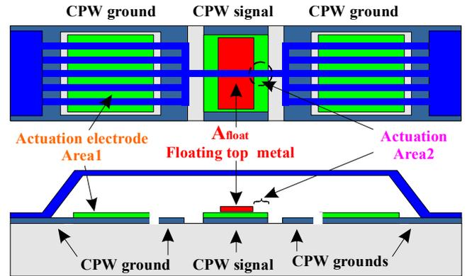
Fig.4: MEMS switch implementing a floating top metal covering the dielectric
