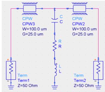
Fig.8: Capacitive shunt switches extraction model
