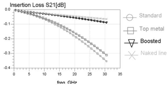
Fig.6a: Simulated HFSS Insertion Loss of standard switch, switch with floating top metal, boosted switch and naked line.
