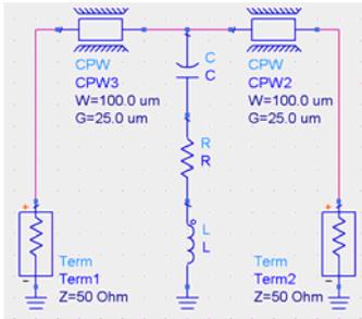
Fig.8: Capacitive shunt switches extraction model
