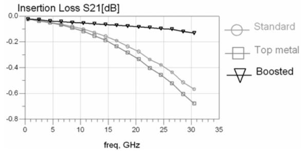
Fig.7a: Insertion Loss measurements
