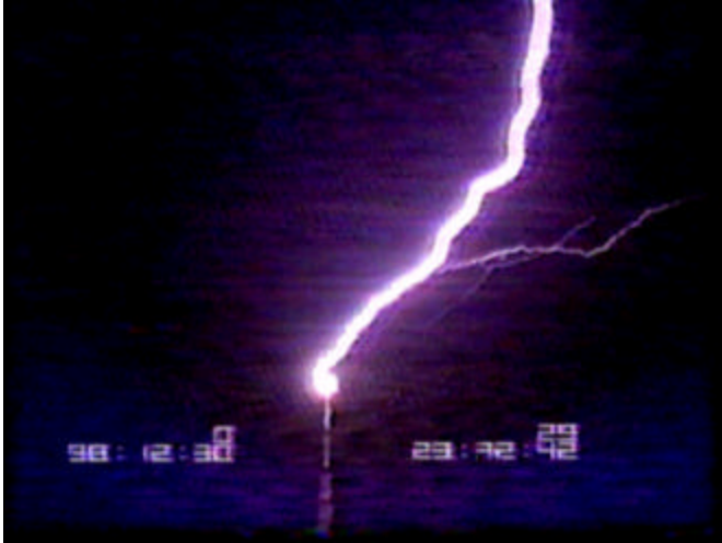
Figure 2. A typical trajectory of a lightning flash striking the tip of the CN Tower.
