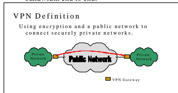
Figure 1: VPN Simplified Schematic Diagram.
