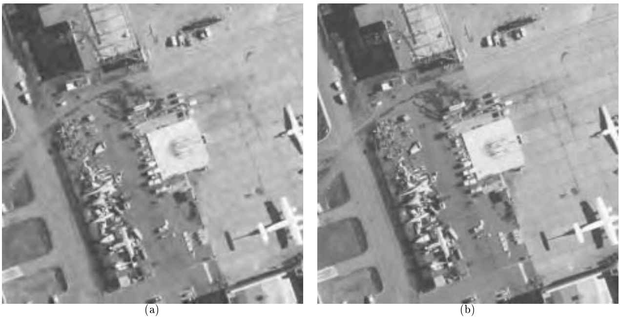
Figure 3: Image Moffett coded at 0.22 bits per pixel using (a) QTCQ (b) our proposed image coder.
