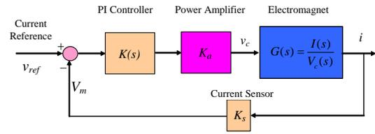
Fig. 5 Closed loop current control system
