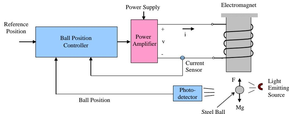
Fig. 1 Magnetic levitation system
