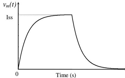
Fig. 3 Step response of the electromagnet
