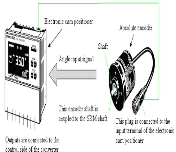
Fig. 3: Connection of the Cam Positioner, Absolute Encoder and Connections.
