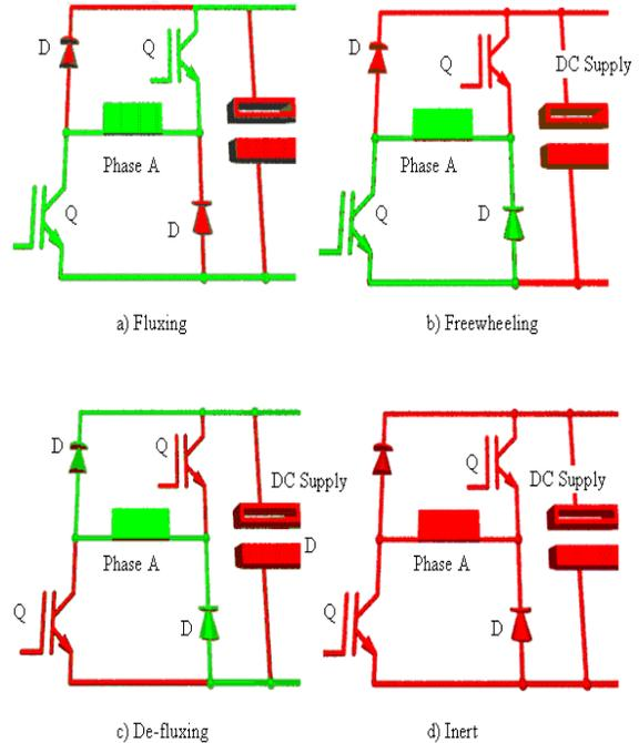
Fig. 2: The Four-Modes of Operation of Classic Converter
