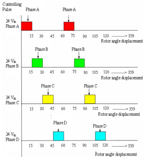
Fig. 6: Firing Angle Sequence of the 4 Phases for Step # 0, and Step # 1.
