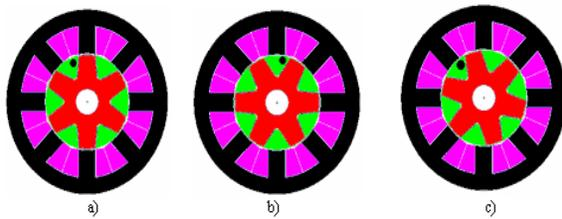
Fig. 5: Structure of an 8/6 SRM: a) Aligned position, b) Unaligned position, c) Misaligned position
