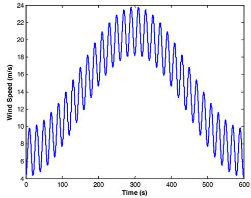
Fig. 4 Wind profile over a period of 10 minutes
