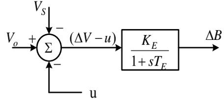
Fig. 6 Block diagram for the capacitance/reactance control
