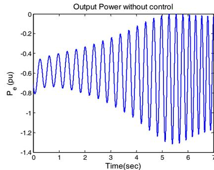
Fig. 10 Power output of the induction generator for 15% torque step without control
