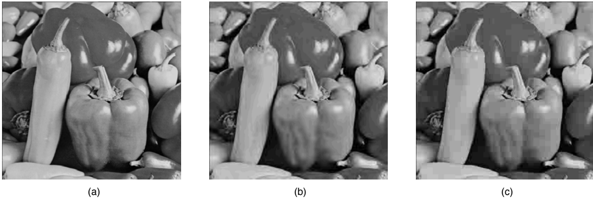
Fig. 5 Performance of the two coding algorithms at scale 4 and 0,125 bits/pixel (a) Original 512x512 8bpp "Peppers" image, (b) PSNR = 29,55 dB (EZW), (c) PSNR = 29,15 dB (EZDCT).
