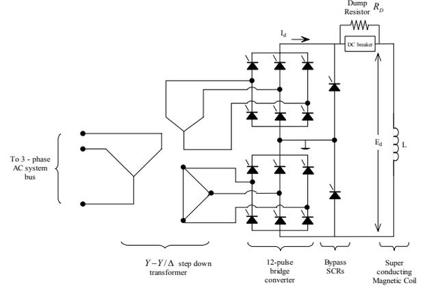
Fig. 2. SMES Circuit point of view
