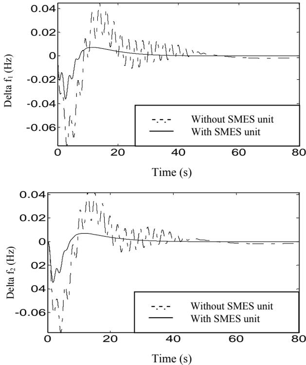
Fig.4: Dynamic responses for area frequencies following the 0.01 pu step load disturbance in area 1
