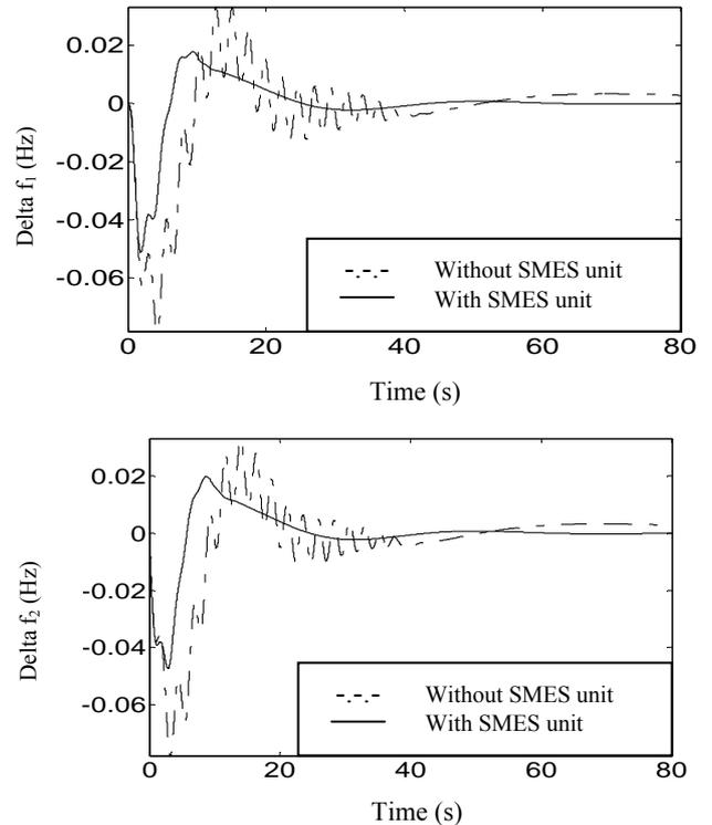
Fig.6: Dynamic responses for area frequencies following the 0.01 pu step load disturbance in area 2
