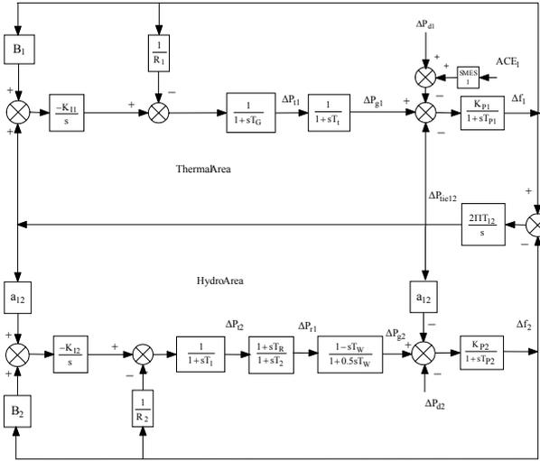
Fig. 1. Two Area Hydrothermal System with SMES unit
