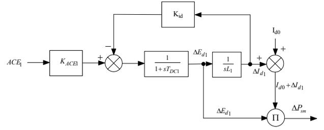
Fig. 3: SMES Block Diagram with Inductor Current Deviation Feedback
