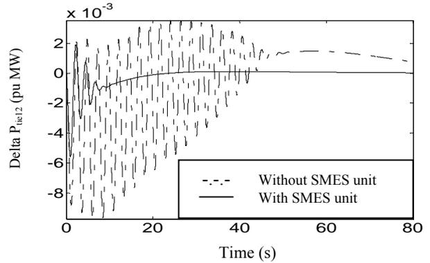
Fig.5: Dynamic response for the tie-power deviation following the 0.01 pu step load disturbance in area 1
