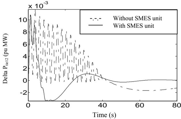
Fig.6: Dynamic responses for the tie-power deviation following the 0.01 pu step load disturbance in area 2
