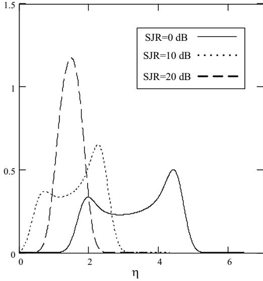
Fig. 2. The pdf of  $\eta$  for various SJRs.
