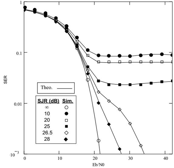
Fig. 6. Analytical and simulated SER performance of FH-MASK for various jamming conditions,  $M = 8$ ,  $q/Q = 0.1$ .
