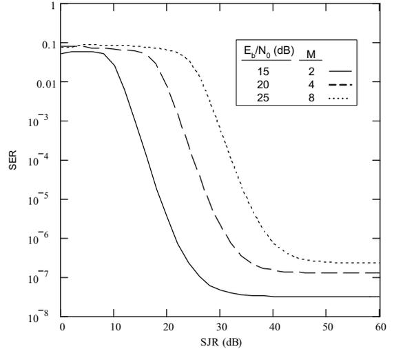
Fig. 7. Analytical SER performance of FH-MASK as a function of SJR for various values of  $E_b/N_0$ ,  $q/Q = 0.1$ .
