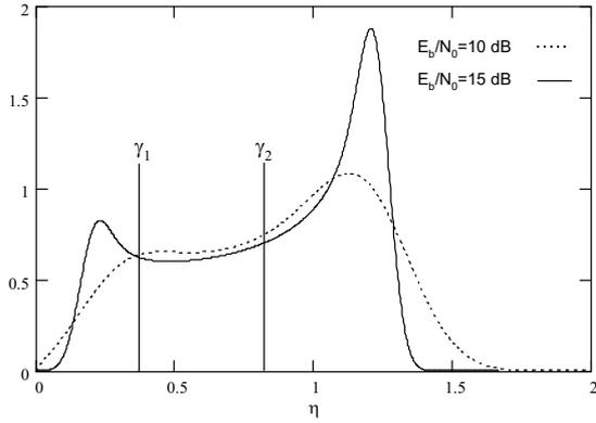
Fig. 4. The pdf of a jammed MASK symbol,  $M = 4$ ,  $i = 1$ , and  $SJR = 10$  dB.
