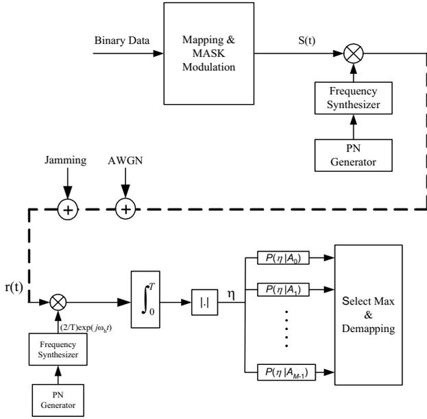
Fig. 1. FHSS-MASK system block diagram
