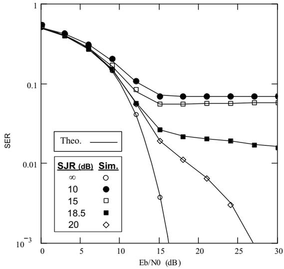
Fig. 5. Analytical and simulated SER performance of FH-MASK for various jamming conditions,  $M = 4$ ,  $q/Q = 0.1$ .
