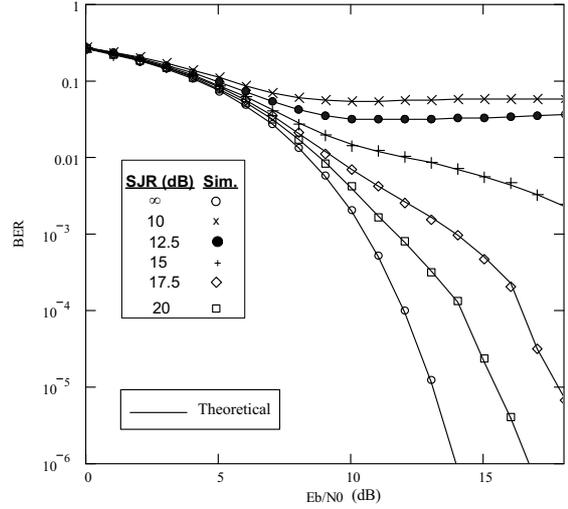
Fig. 3. Analytical and simulated BER performance of FH-MASK for various jamming conditions,  $M = 2$ ,  $q/Q = 0.1$ .
