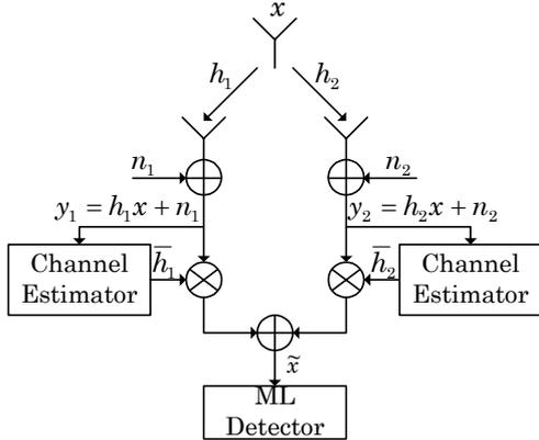
**Figure 1:** Baseband representation of the MRC technique using two receivers.
