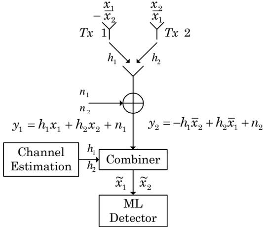
**Figure 2:** Simple two-transmitter STB code  $\mathbf{G}_2$  using one receiver.
