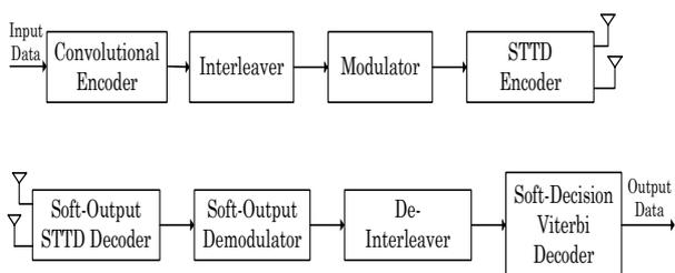
**Figure 3:** A block diagram of the concatenated system.
