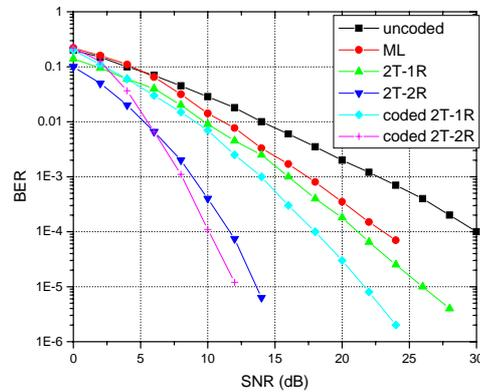
**Figure 5:** BER curves of convolutional-coded system with transmit and receive diversity.
