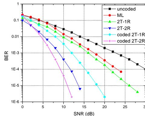
**Figure 7:** BER of turbo-coded system with transmit and receive diversity using Log-MAP.
