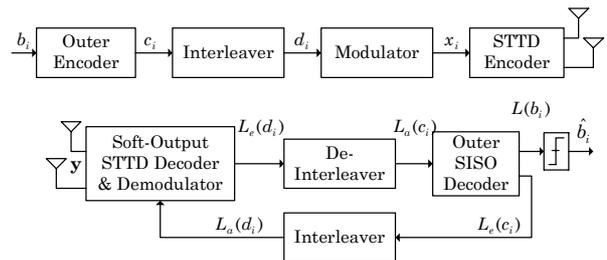
**Figure 4:** Iterative detection and decoding for a system with transmit diversity.
