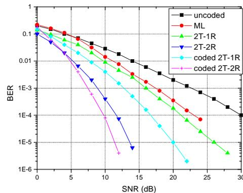
**Figure 6:** BER of turbo-coded system with transmit and receive diversity using SOVA.
