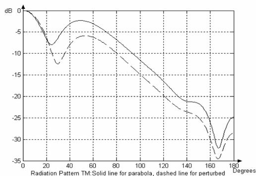
Fig. 1 Radiation pattern (TM) of parabolic and perturbed parabolic for the following parameters:  $L=1$ ,  $f=0.7$ ,  $R=0.05$ ,  $d_1=d_2=f$
