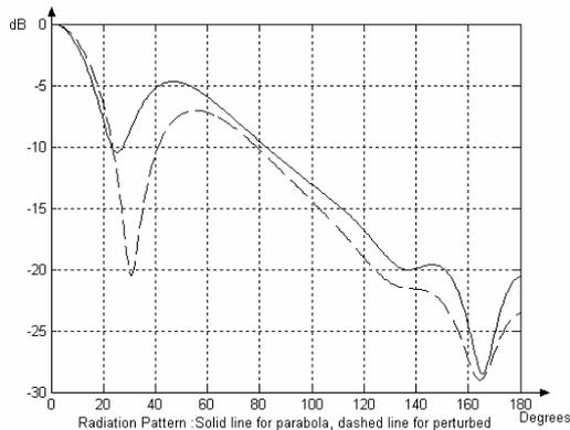
Fig. 2 Radiation pattern (TE) of parabolic and perturbed parabolic for the following parameters:  $L=1$ ,  $f=0.5$ ,  $R=0.2$ ,  $d_1=d_2=f$ .
