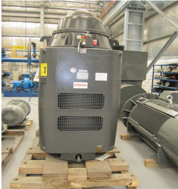
Figure 4 : Vertical motor with 100 hp,480 V,3565 rpm
