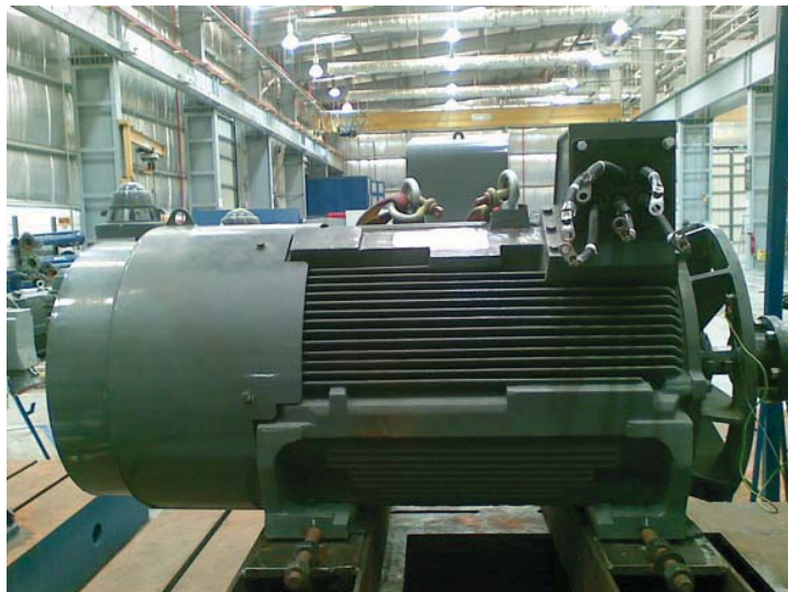
Figure 3 : AC motor with 400 hp,480 V,3570 rpm
