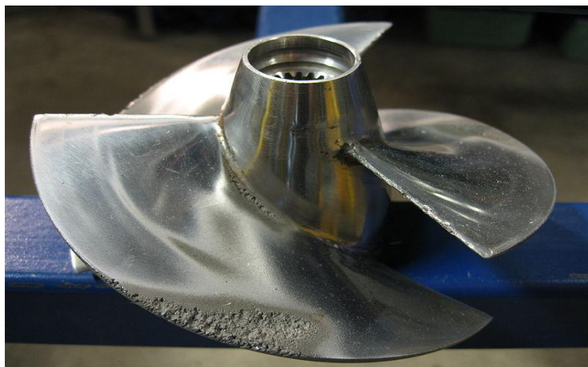
*The cavitations are clear on the impeller*
