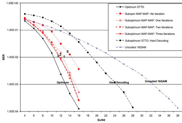
Figure 3: Performance of the 4b/s/Hz STT coded two-group system using the Suboptimum MAP-MAP Joint STTDs over  $4 \times 2$  MIMO quasi-static Rayleigh fading channels.
