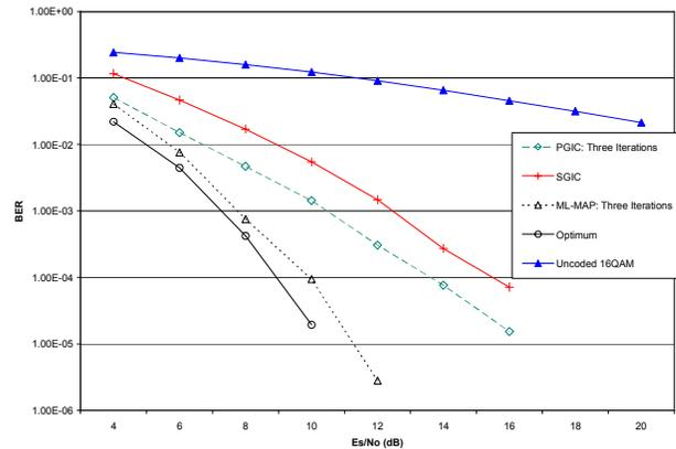
Figure 6: Performance comparison of the 4b/s/Hz STT coded two-group receivers. The channel is a  $4 \times 4$  MIMO quasi-static Rayleigh fading channel.
