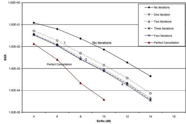
Figure 5: Performance of the 4b/s/Hz STT coded two-group system using the PGINC receiver. The channel is a  $4 \times 4$  MIMO quasi-static Rayleigh fading channel.
