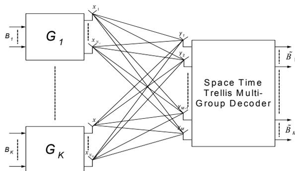
Figure 1: Block Diagram Of the Multi-Group Space Time Trellis Coding architecture
