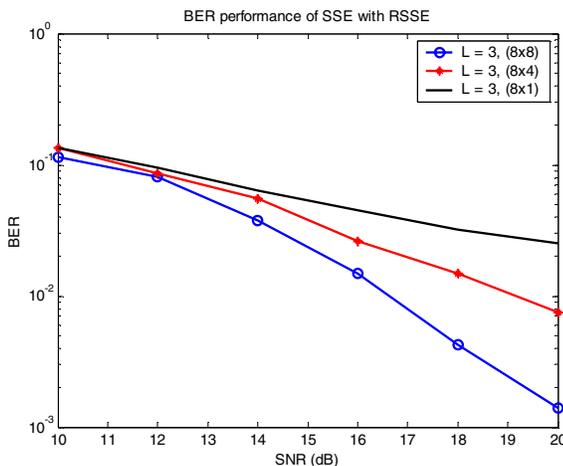
Figure 3: BER performance of SSE with RSSE, 8PSK,  $N_T = N_R = 6$ .
