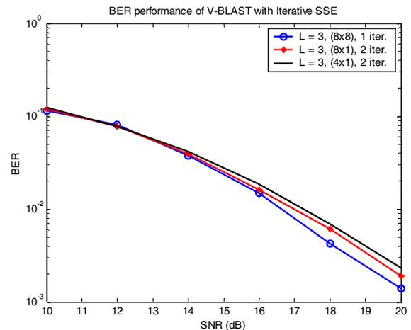
Figure 4: BER performance of iterative SSE with 8PSK,  $N_T = N_R = 6$ .
