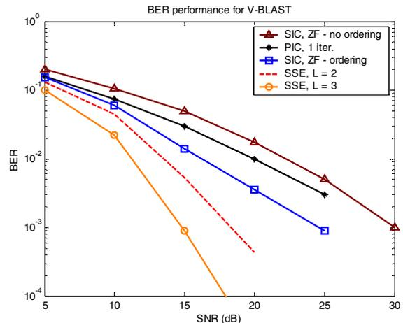
Figure 2: Performance comparison for different V-BLAST algorithms with QPSK,  $N_T = N_R = 4$ .
