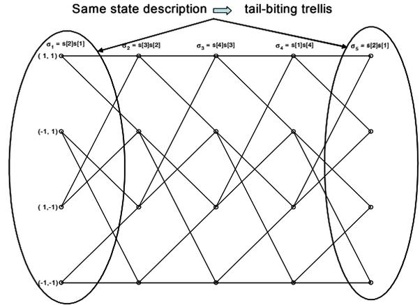
Figure 1: SSE trellis diagram for BPSK,  $N_T = 4, L = 3$ .
