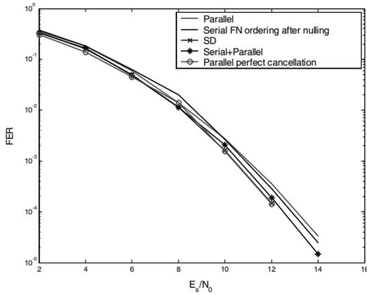
Figure 5: MLSTBC-OFDM at 4bps/Hz,  $K=2$ ,  $M_R=4$  and  $N_T=2$  antennas per group
