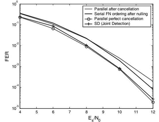
Figure 7: MLSTBC-OFDM at 8bps/Hz,  $K=4$ ,  $M_R=8$  and  $N_T=2$  antennas per group
