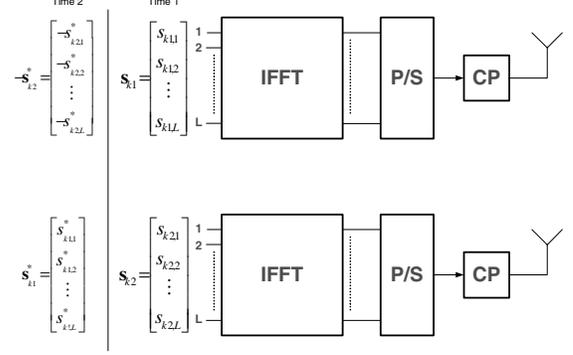
Figure 2: Architecture of a single STBC-OFDM transmitter.
