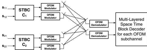
Figure 1: Block diagram of MLSTBC-OFDM.
