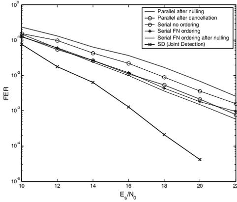
Figure 4: MLSTBC-OFDM at 4bps/Hz,  $K=2$ ,  $M_R=2$  and  $N_T=2$  antennas per group
