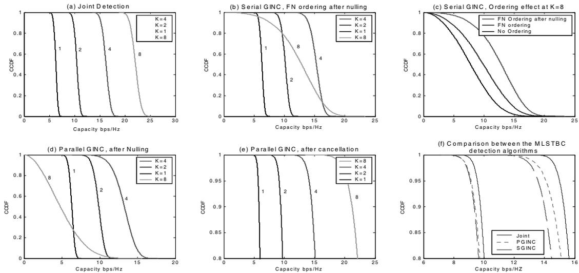
Figure 3: Capacity CCDF of MLSTBC detection algorithms.
