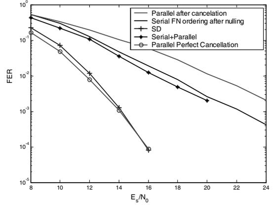
Figure 6: MLSTBC-OFDM at 8bps/Hz,  $K=4$ ,  $M_R=4$  and  $N_T=2$  antennas per group
