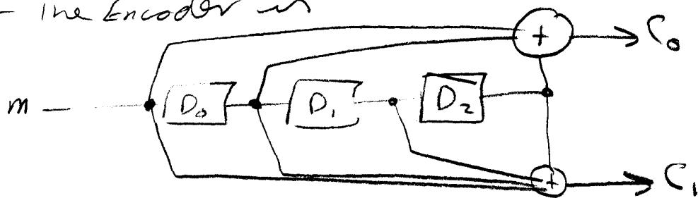
The Memory depth  $M = \text{Mat deg}(g_0, g_1)$
