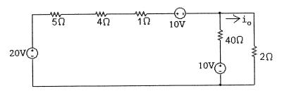
Now combine the 20 V and 10 V sources into a single voltage source and the 5  $\Omega$ . 4  $\Omega$  and 1  $\Omega$  resistors into a single resistor to get
