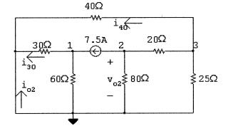
$$\frac{v_2}{80} + 7.5 + \frac{v_2 - v_3}{20} = 0$$
