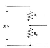
Maximum dissipation in  $R_2$  occurs at no load, therefore,
