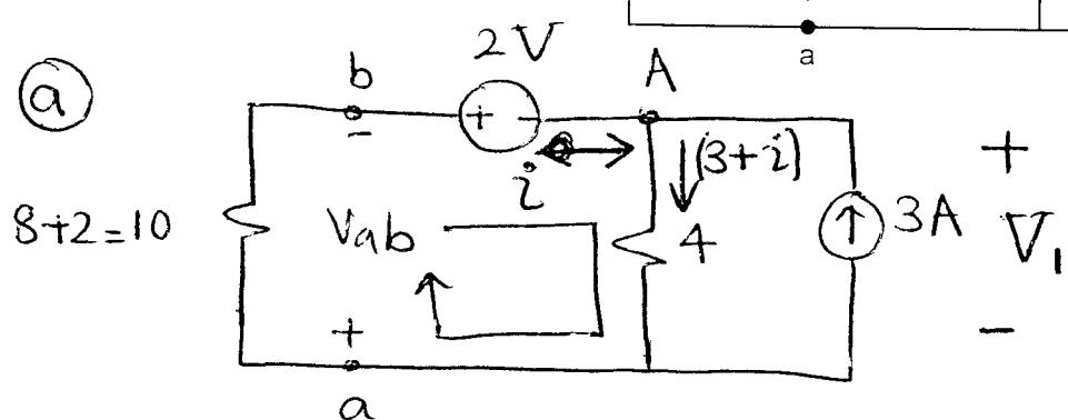
Apply KVL in the left loop after applying KCL at A.
