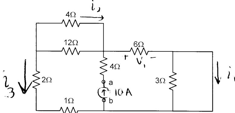
Since  $3\Omega$  is in parallel to a short ckt it can be removed.
