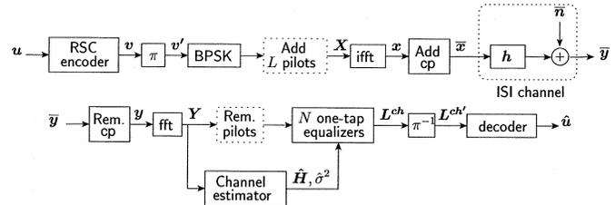
Fig. 1. Coded OFDM system model.
