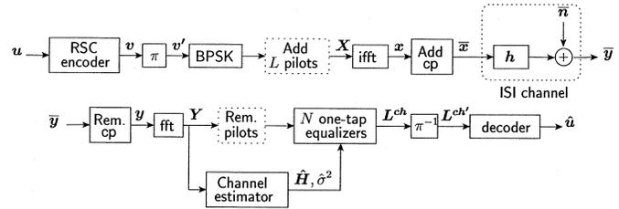
Fig. 1. Coded OFDM system model.
