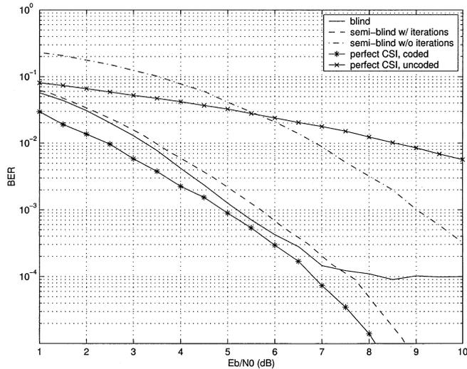
Fig. 3. BER versus  $E_b/N_0$  for the various systems.
