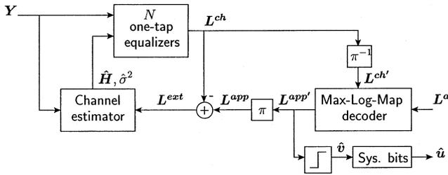
Fig. 2. Iterative decoding and channel estimation.
