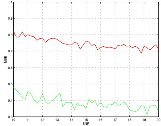
Figure 3: Reduction in MSE due to EM iterations– steady-state MSE vs. SNR before and after invoking the EM iterations
