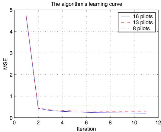
Figure 1: Reduction in MSE due to pilot overhead– EM learning curves for different number of pilots
