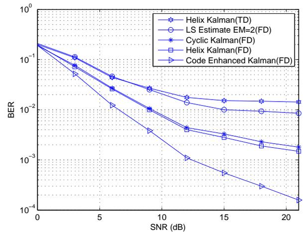
**Fig. 2.** BER comparison of entire system (TD: Time Domain, FD: Frequency Domain).
