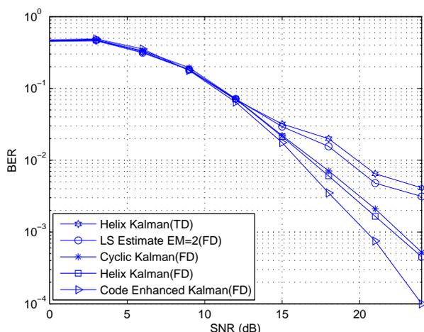
**Fig. 3.** BER comparison for correlated case (TD: Time Domain, FD: Frequency Domain).
