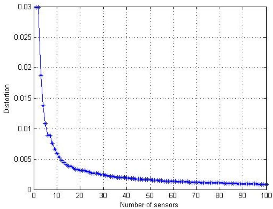
Figure 2: Average distortion for varying number of sensor nodes.
