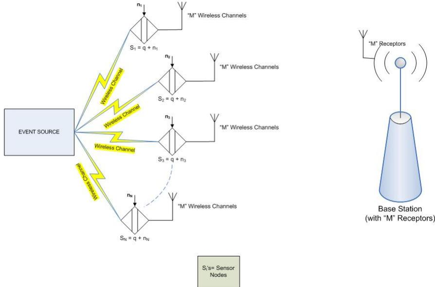
Figure 1: The wireless sensor network mode.
