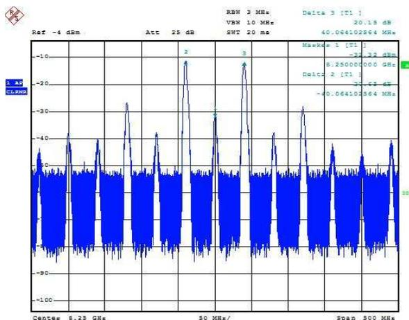
Figure 9: Spectrum of the Modulator
