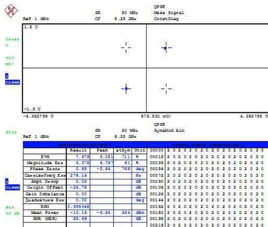
The figure above shows that after integration with the power amplifier the value of EVM degrades from 0.543% to 7.479% but still the value is under the desirable range. For most of the transmitter studied it has been observed that EVM has to be kept lower than 20%. If the value of EVM is under 20% then the design of the modulator is quite efficient. This is because the value of EVM for whole transmitter is dependent on the modulator. The better the EVM of the
