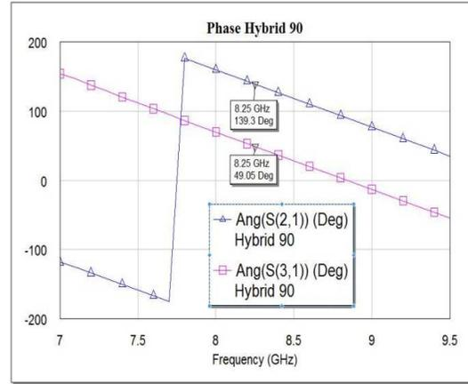
Figure 5: Phase of Branch Line Coupler
