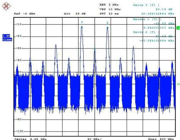
Figure 9: Spectrum of the Modulator
