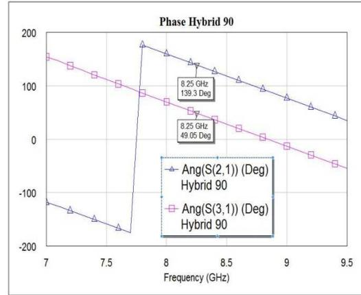
Figure 5: Phase of Branch Line Coupler
