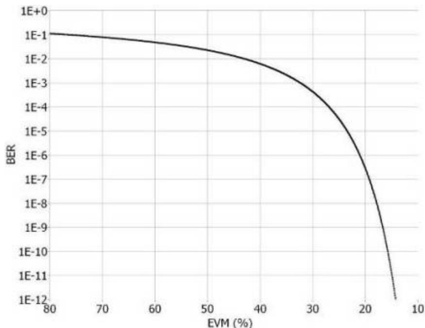
Figure 12: BER vs. EVM of QPSK [9]
