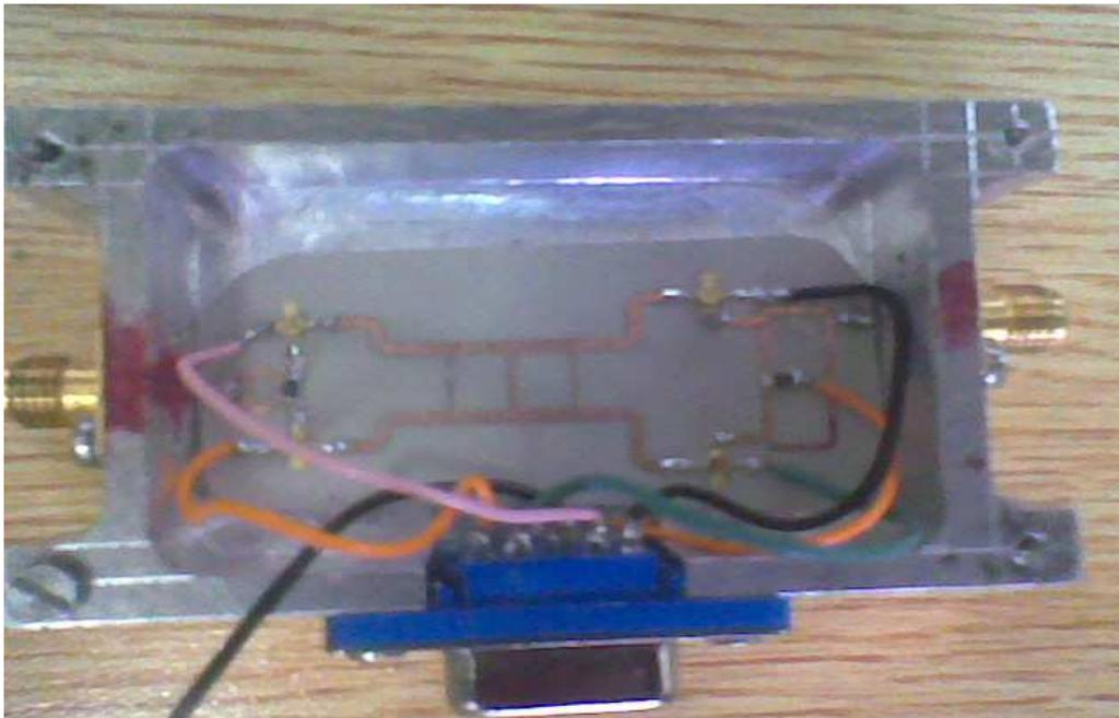
Figure 11: Hardware of the Modulator
