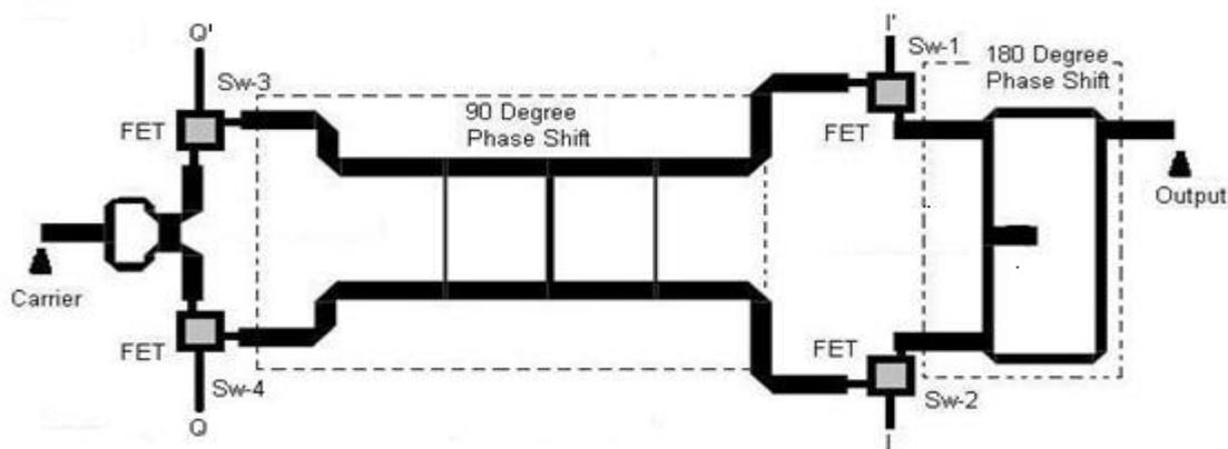
Figure 1: The Design of QPSK Modulator
