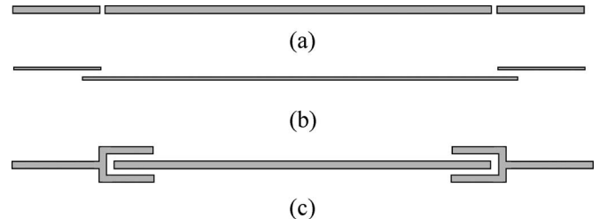
Fig. 1. Resonator configurations with three types of feeds. (a) Microstrip resonator with feed parts as short microstrip lines separated by small gaps from the resonant segment (top view). (b) Stripline resonator with feed parts as short microstrip lines overlapping the resonant segment (side view). (c) Microstrip resonator with fork-shaped feed configuration (top view).
