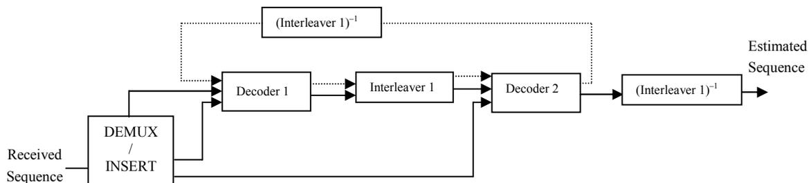
Figure 2. Block diagram of a turbo decoder.
