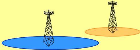
For Coverage, CDMA saves wireless carriers from deploying the 400% more cell site that are required by GSM
