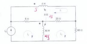
c) Write a set of mesh-current equations that describe the circuit in terms of the currents  $i_1$  and  $i_2$  in the frequency domain, where the source current,  $i_g$ , is known and it has  $\omega = 0.25$  rad/s. (Hint: first represent in the  $j\omega$  domain)
