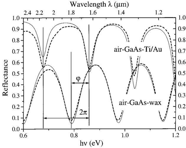
Fig. 16. Measured and calculated reflectivity of metal clad (air-GaAs-Ti/Au) and dielectric clad (air-GaAs-wax) F-P cavities: reflectance that we calculated using the transfer matrix method, solid curves; experimental curves from Ref. 77, dashed curves.
