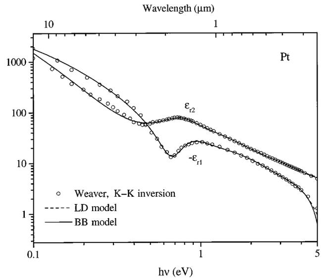
Fig. 9. Real and imaginary parts of the optical dielectric function of Pt versus photon energy (open circles, data from Weaver<sup>64</sup>; solid curves, BB model; dashed curves, LD model).
