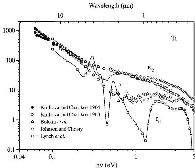
Fig. 10. Real and imaginary parts of the optical dielectric function of Ti: experimental data points, Kirillova and Charikov,<sup>72,73</sup> Bolotin *et al.*,<sup>74</sup> Johnson and Christy,<sup>61</sup> and Lynch *et al.*<sup>70</sup>
