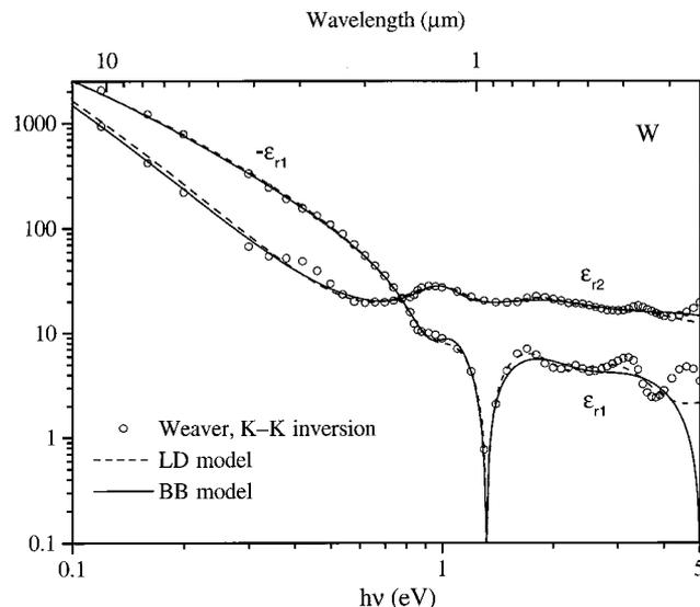
Fig. 12. Real and imaginary parts of the optical dielectric function of W versus photon energy (open circles, data from Weaver *et al.*<sup>75</sup>; solid curves, BB model; dashed curves, LD model).
