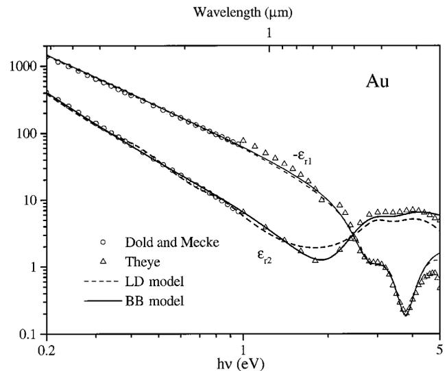
Fig. 2. Real and imaginary parts of the optical dielectric function of Au: solid curves, values that we calculated using the BB model; dashed curves, the LD model. Also shown are selected experimental data points from Dold and Mecke<sup>46</sup> and Thèye.<sup>49</sup>
