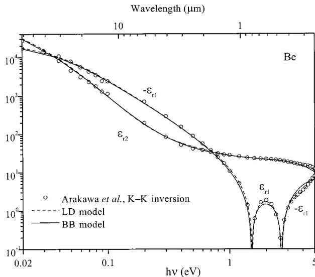
Fig. 5. Real and imaginary parts of the optical dielectric function of Be versus photon energy (open circles, data from Arakawa *et al.*<sup>57</sup>; solid curves, the BB model; dashed curves, the LD model).
