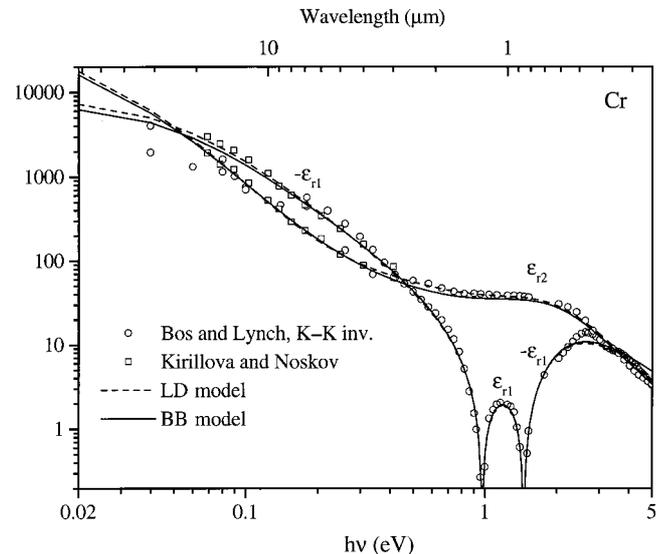
Fig. 6. Real and imaginary parts of the optical dielectric function of Cr: solid curves, values that we calculated using the BB model; dashed curves, the LD model. Also shown are tabulated data from Bos and Lynch<sup>58</sup> and Kirillova and Noskov.<sup>60</sup>
