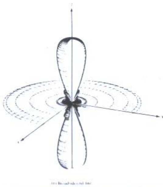
Figure 6.6 Three-dimensional amplitude patterns for broadside, and broadside/end-fire arrays.
